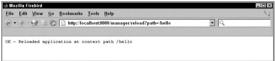
Figure 7-8: Reloading a Web application.
