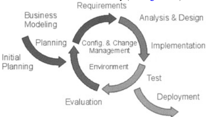
Figure 3.3: RUP cycle. Source: Life Cycles of the Rational Unified Process. Reprinted with permission.
