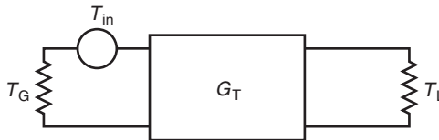
FIGURE 11.19 Noise within the circuit is referred to the input side.
