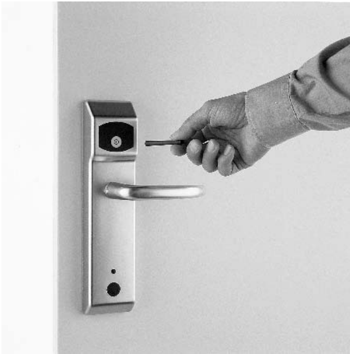
Figure 13.17 Offline terminal integrated into a doorplate. The lock is released by holding the authorized transponder in front of it. The door can then be opened by operating the handle. The door terminal can be operated for a year with four 1.5 V Mignon batteries and even has a real time clock that allows it to check the period of validity of the programmed data carrier. The terminals themselves are programmed by an infrared data transmission using a portable infrared reader (reproduced by permission of Häfele GmbH, D-Nagold)
