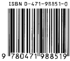
Figure 1.3 Example of the structure of a barcode in EAN coding
