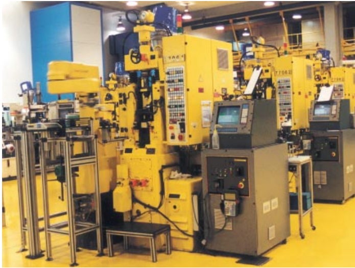
Fig. 4.1-18 Pressing setup with a controlled process and an automatic handling system
