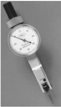
Fig. 3.1-7 Dial gage, comparator dial, and lever-type test indicator (courtesy: Mahr)
