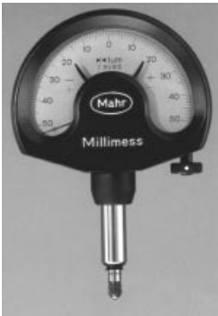
Fig. 3.1-7 Dial gage, comparator dial, and lever-type test indicator (courtesy: Mahr)
