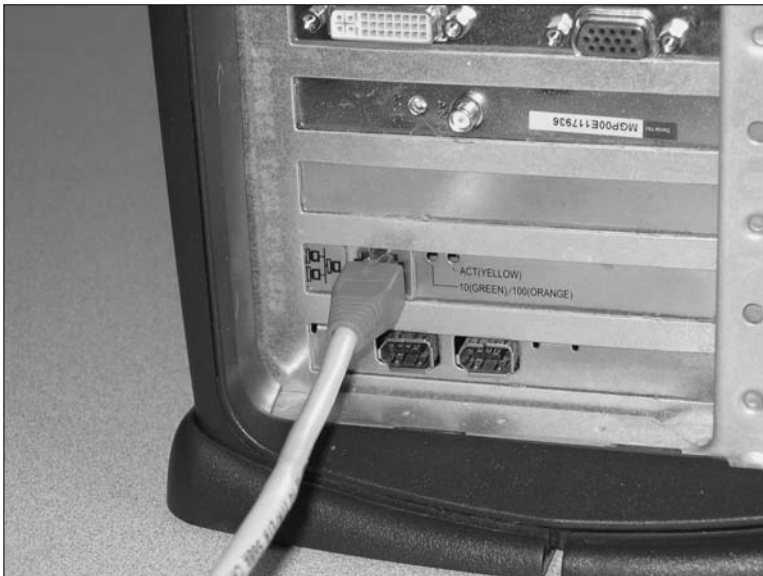
Figure 10-1: Connecting Ethernet cable to PC Ethernet port
