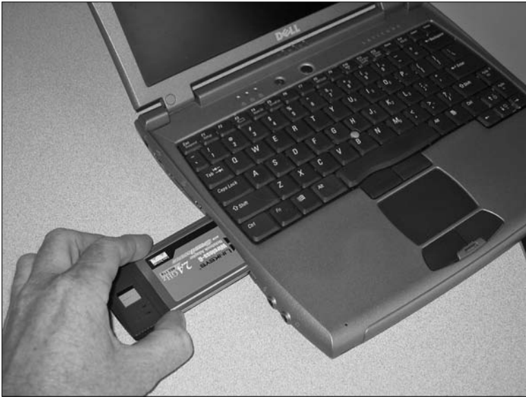
Figure 13-3: Inserting a wireless card into a notebook
