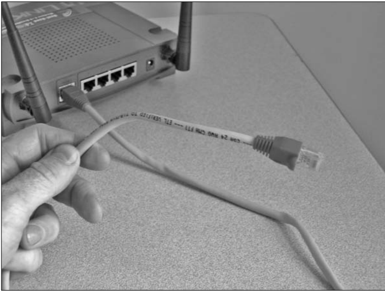
Figure 12-9: Connecting Ethernet cable to a wireless router
