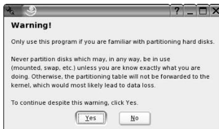
Figure 14-3: YaST's partitioning warning
