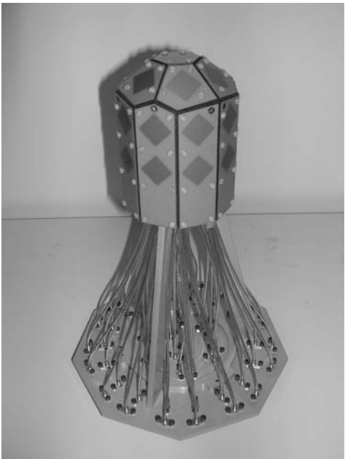
Figure 6.37 3-D Dual-polarized antenna array for 5.25 GHz. Source: Elektrobit Testing Ltd.
