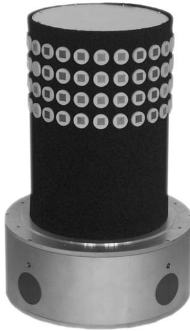
Figure 6.40 Stacked polarimetric uniform circular patch array (SPUCPA 4 \times 24 ). Source: Technische Universität Ilmenau.
