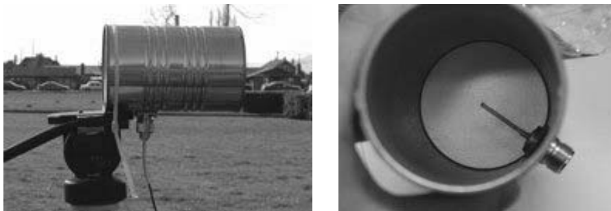
Figure 9.10 Tin-can wireless antenna.
