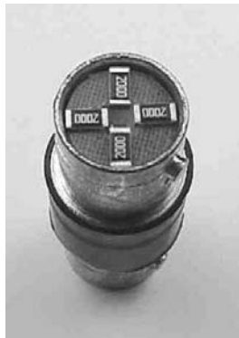
Step 1c Washer and resistors inserted into the BNC connector.
