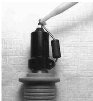
Figure A.17 FET probe shorted by its ferrite equipped ground lead.
