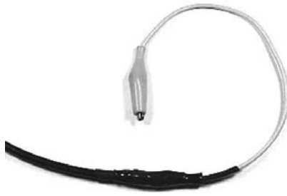
Figure A.11 Resistive current probe.
