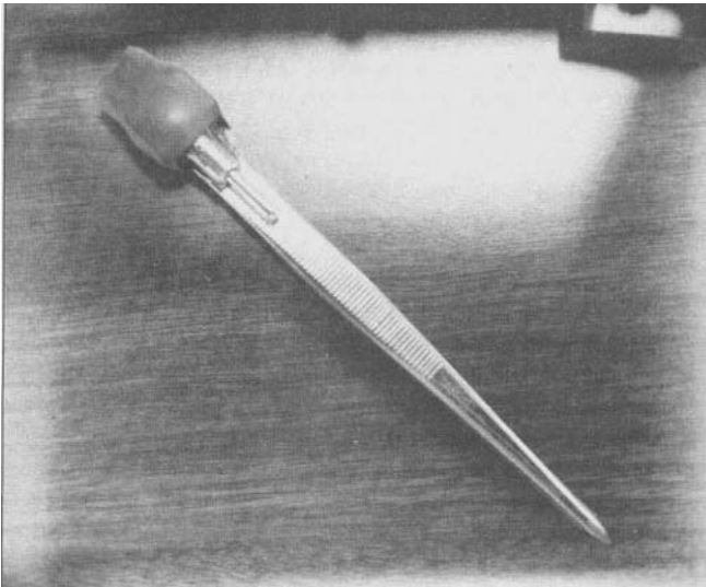
Figure 9.20 Fully manufactured tweezer probe assembly. (Switch is provided for switching in discrete components.)
