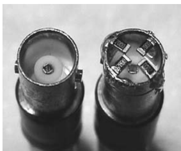
Step 1a 50-ohm termination.
