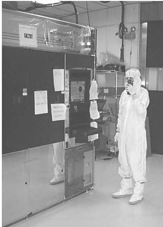
Figure B.14 Radiated immunity testing with hand-held radio in a semiconductor manufacturing clean room.
