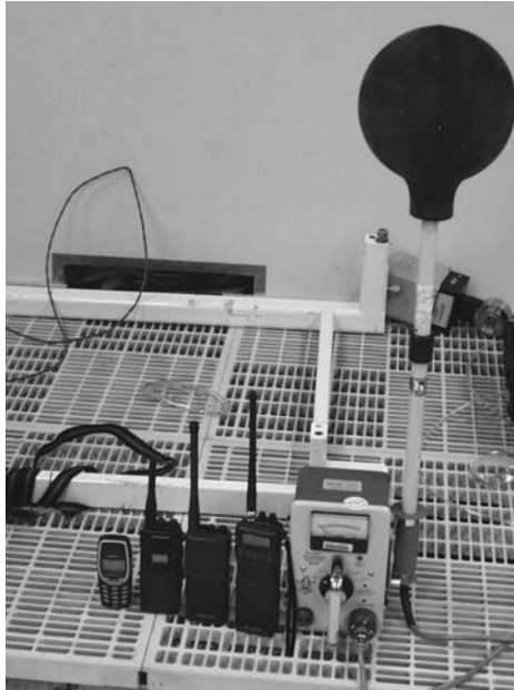
Figure B.12 Hand-held radios and field intensity meter.
