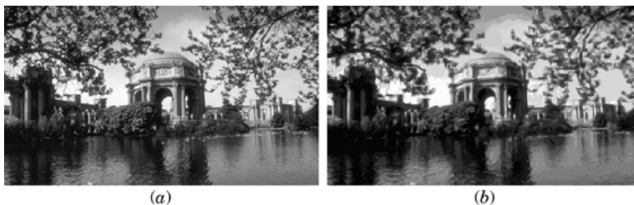
Figure 10.2 Demonstration of ABC-simulated retinal image of typical scene, including (a) original (DR = 1:1) and (b) ABC-reconstructed image with a = 0.016 and DR = 20:1. Catastrophe-resolving element, a , is defined as fraction of total scene horizontal size. Data-reduced image (b) has been obtained by applying only second (singular) term of Eq. 10.2, with linear approximation between singularities. Photometric term contribution can be recognized here as difference: (a) – (b). This means that ABC algorithm filters image entirely on basis of two catastrophes: cusp and fold . This seems analogous to foveal fixation points. Red square in corner illustrates size of catastrophe-resolving element, a .
