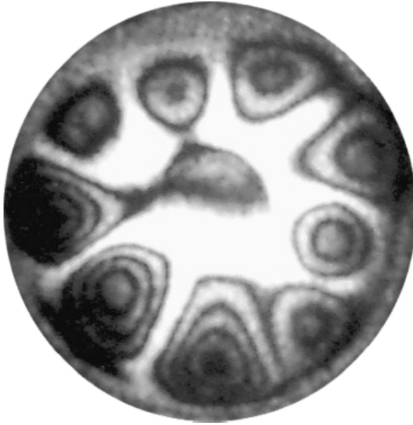
Figure 3.16 Photograph of real-time holographic pattern of vibrating membrane in self-stabilized holographic recording in BTO photorefractive crystal in pure diffusion regime. Bright regions correspond to vibration nodes.
