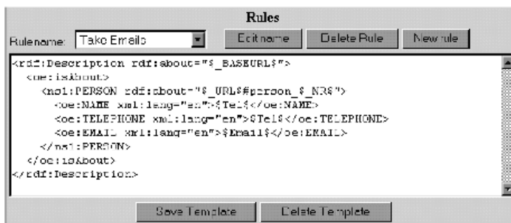
Figure 6.4 Template defining an instance of class 'person' used by OntoWrapper
