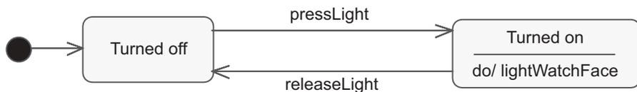
Figure 6.11 State diagram for managing the light
