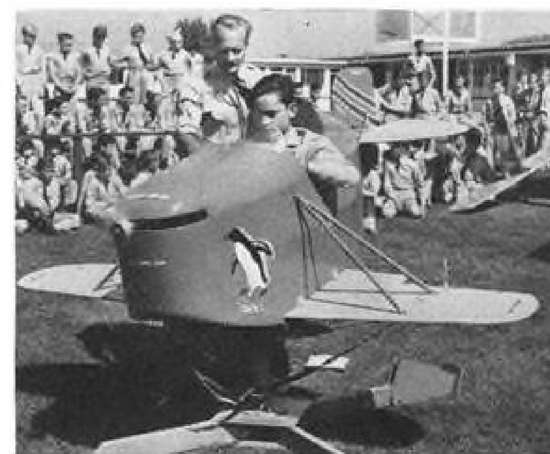
Classroom Trainer: Volmer Jensen, chief engineer of California Aero Glider Co., explains operation of company's classroom trainer. Not shown are the trainer's instrument-flight hood and earphone remote instruction equipment.
