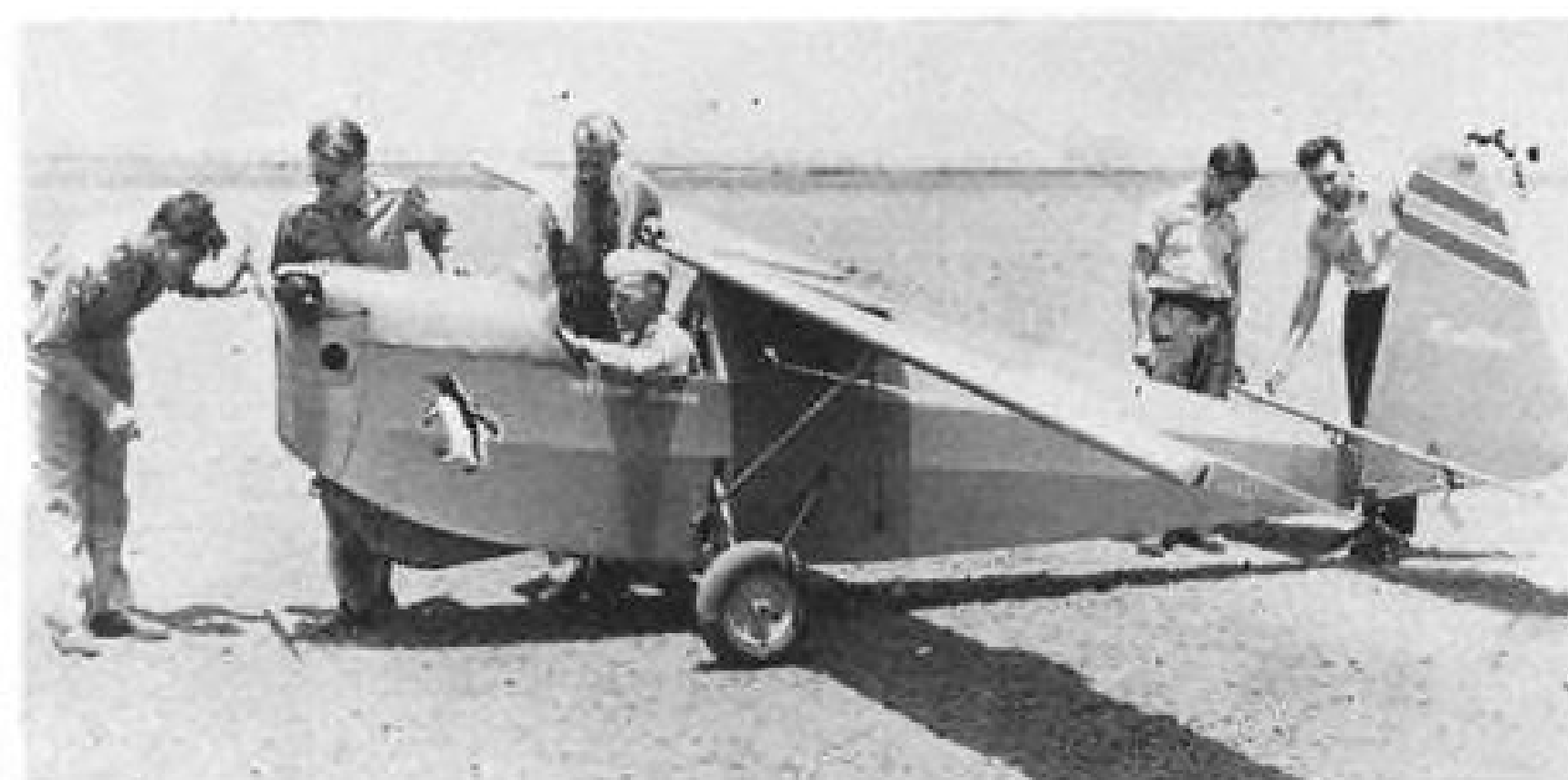
Parody, vice-president, is in cockpit. On right is a motorized advanced pre-flight trainer which aroused the Army's interest and won an experimental contract. Controls are sensitive at 5 mph. Top speed is 40 mph.
