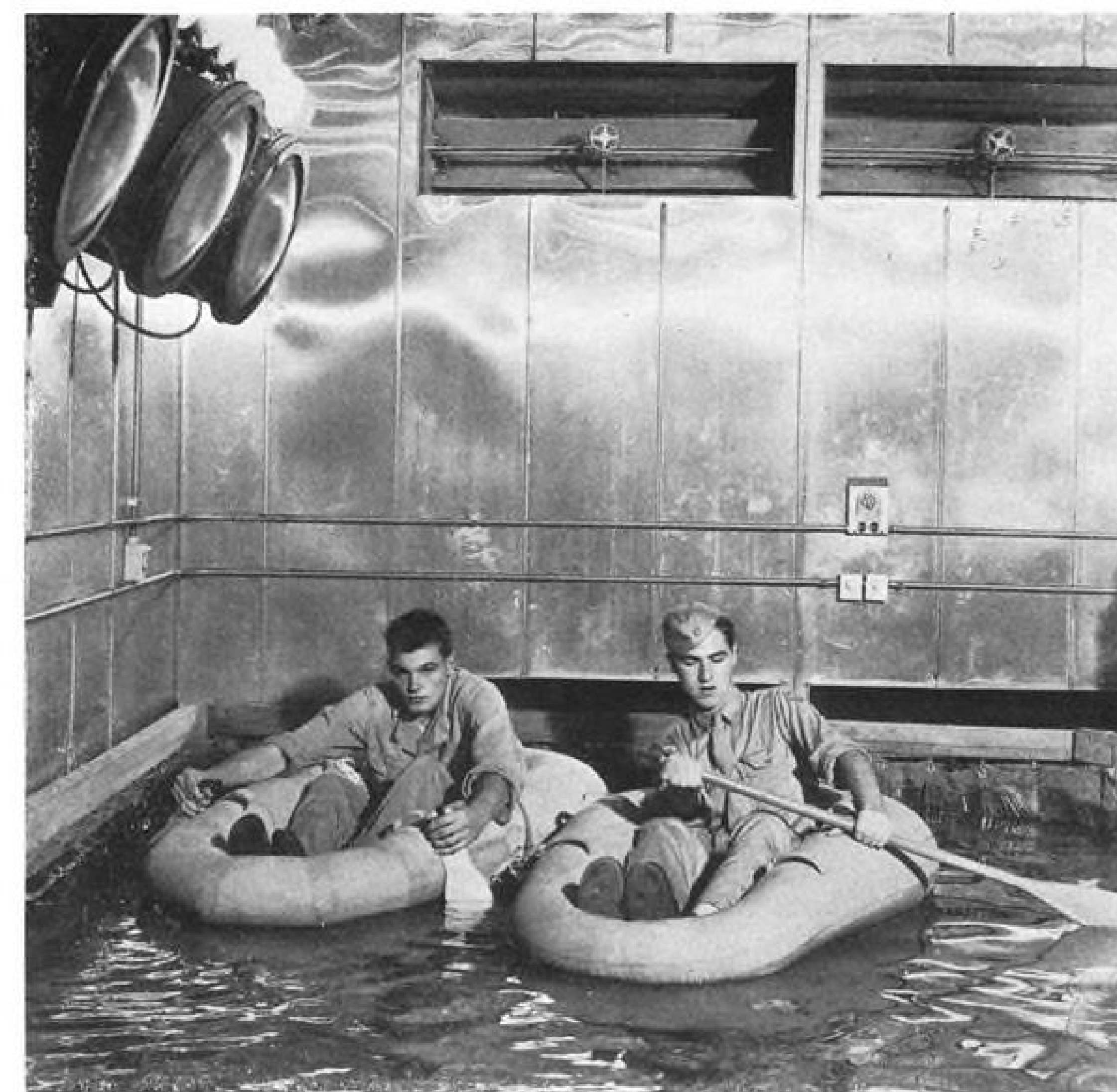
Wright Field's New All-Weather Chamber: can test Army equipment developed for use in any climate. It can reproduce artificially, hail storms, rainstorms, sand storms, sleet, fog, jungle humidity, temperatures as low as 60 below zero and as high as 150 degrees above zero. Above: Two Aero-medical laboratory soldiers paddle their one-man life rafts in the chamber to test water emergency equipment. The big lights along the left wall are 1,500-watt sun lamps, which in combination with the smaller ultra-violet ray lamps, produce artificial sunlight. Cold air, to simulate Arctic conditions, comes in through the vents in the wall behind the men.
