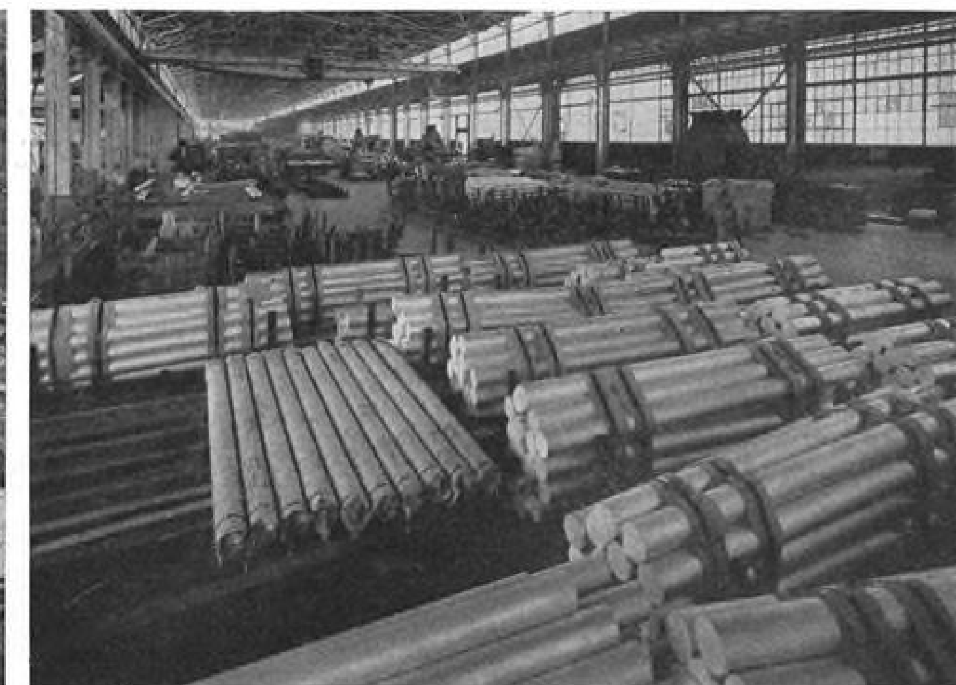
Reynolds rolled aluminum alloy forging stock, tested and Army-Navy inspected, ready to be forged into aircraft propellers.
