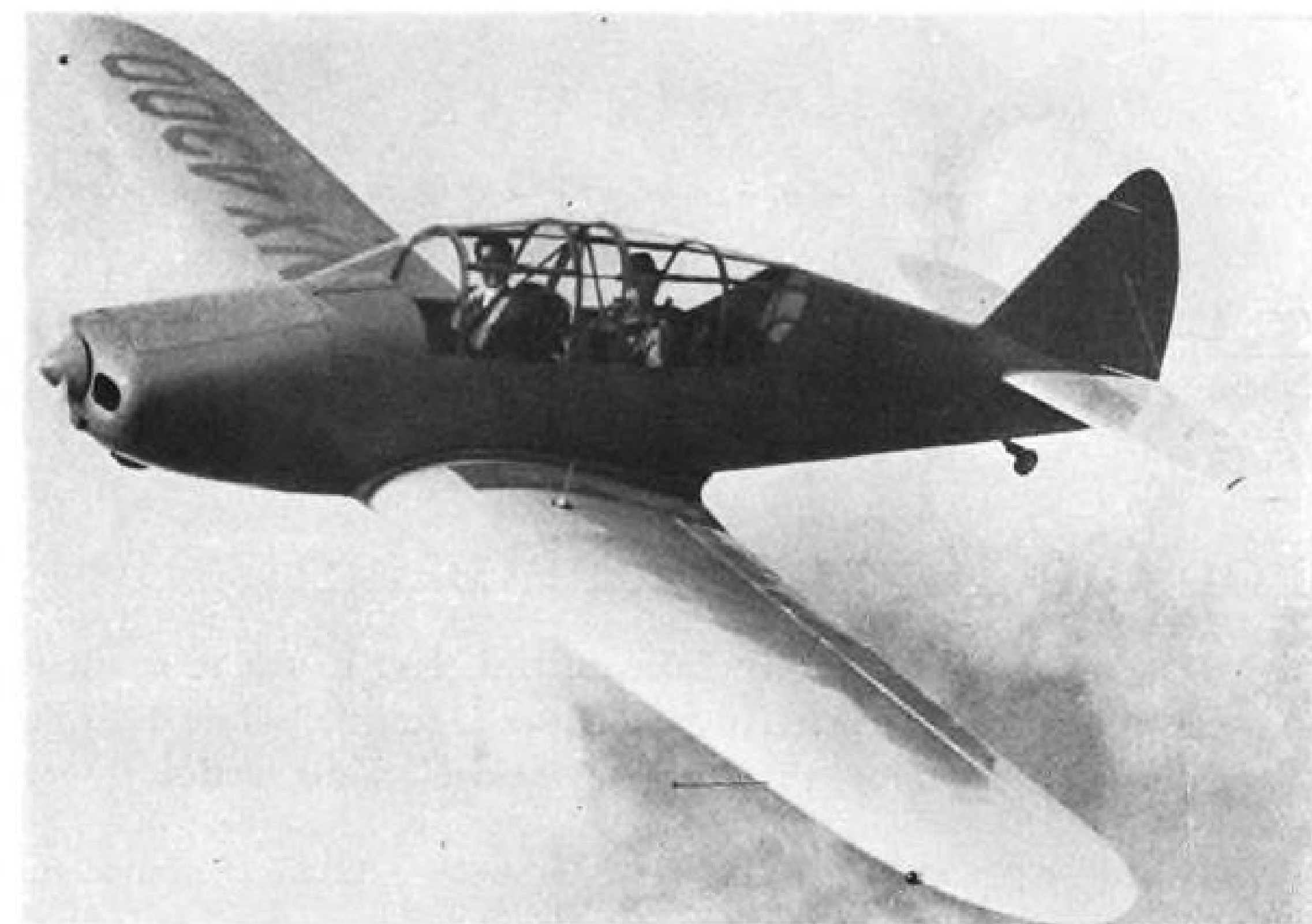
New Piper PT Experimental Plane: This new low-wing model, shown in flight and on the ground, is designed for multi-purpose duty, with excellent vision for both instructor and student. Non-strategic materials are used wherever possible. It is powered by a six-cylinder, 130-hp. Franklin engine.
