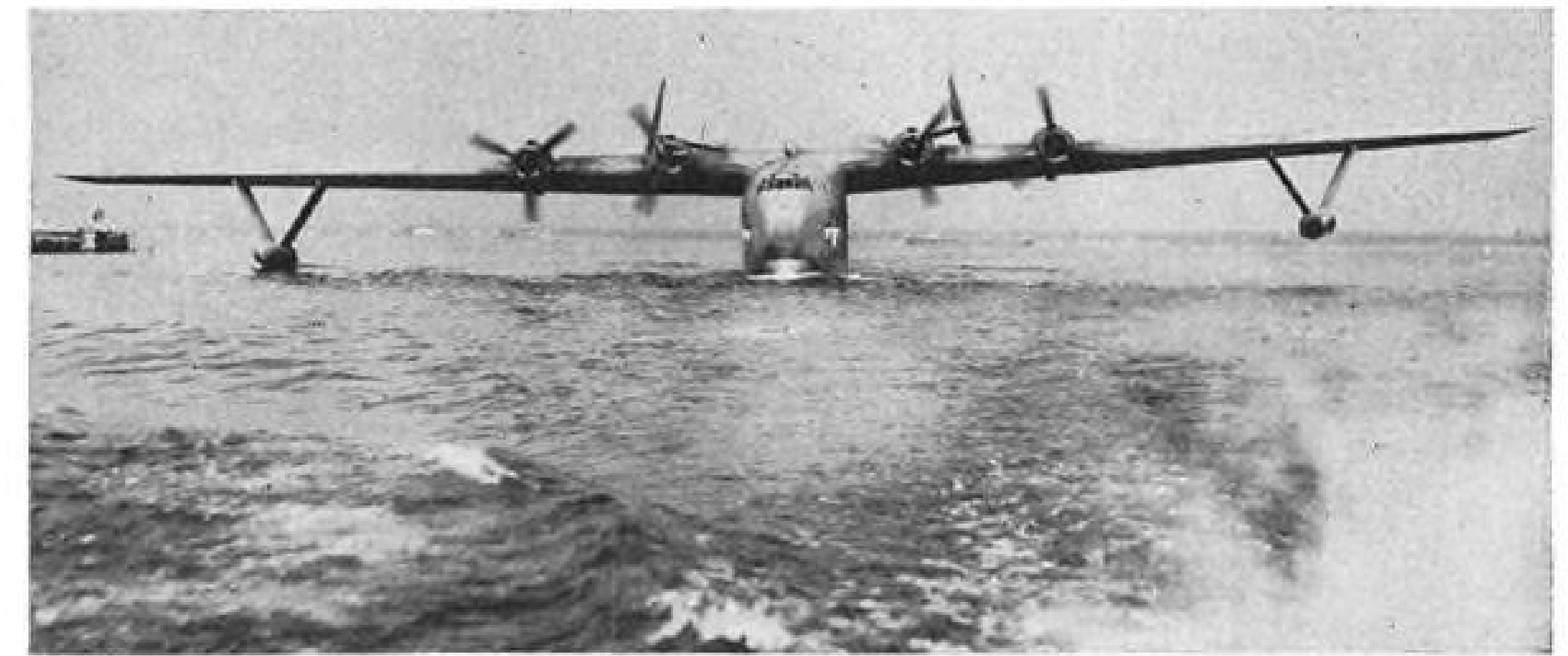
Shatters Aerial Records: On her first war mission, the giant Mars, Naval Air Transport Service's new cargo flying boat, shattered four world's records on the Patuxent River, Md., to Natal, Brazil, non-stop flight of 4,375 miles and the return journey by stages. The Mars took off from Patuxent weighing 148,500 pounds gross, the heaviest weight ever lifted by a plane.
