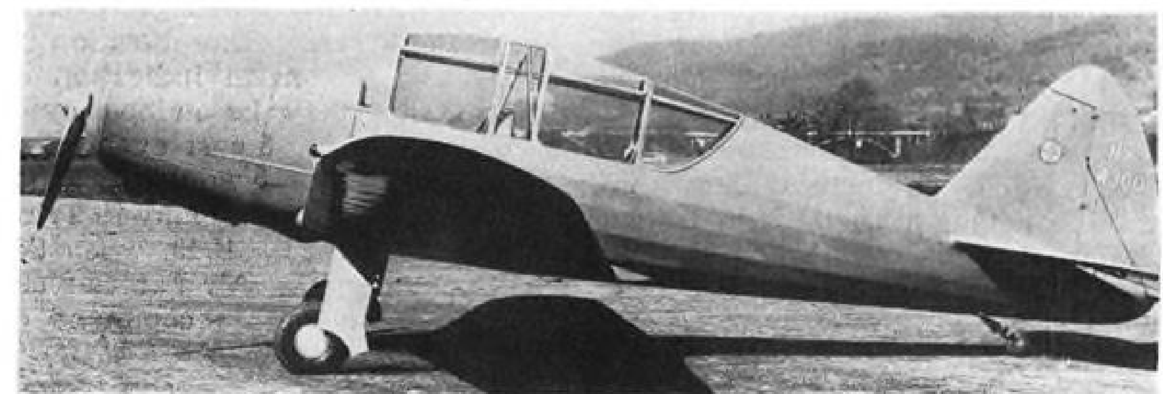
New Piper PT Experimental Plane: This new low-wing model, shown in flight and on the ground, is designed for multi-purpose duty, with excellent vision for both instructor and student. Non-strategic materials are used wherever possible. It is powered by a six-cylinder, 130-hp. Franklin engine.
