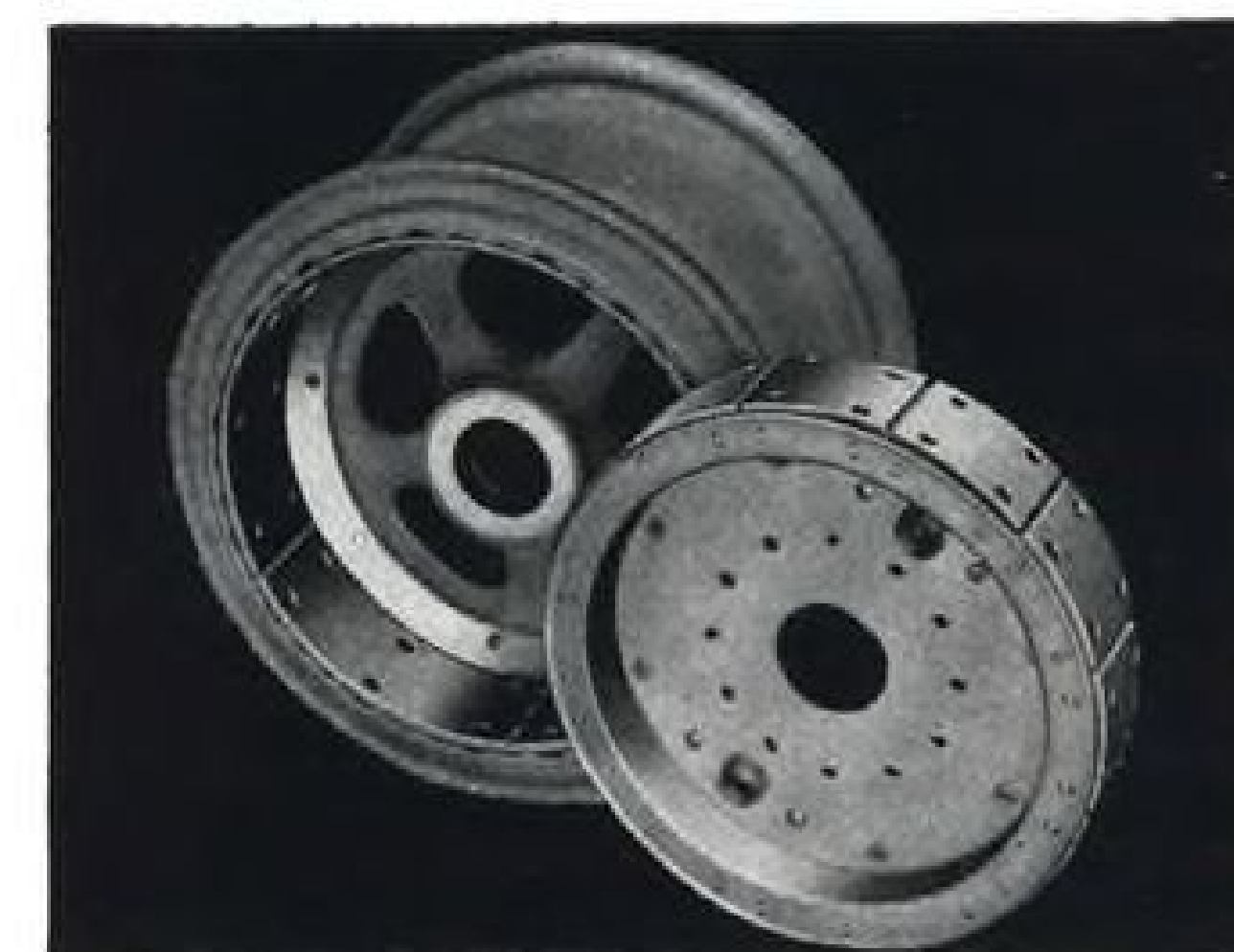
The GENERAL 9 x 12 Expander-Tube Brake and Wheel— Partially Assembled . Remember, you can depend on General for longer service life . . . simpler maintenance . . . easier, "softer" operation!
