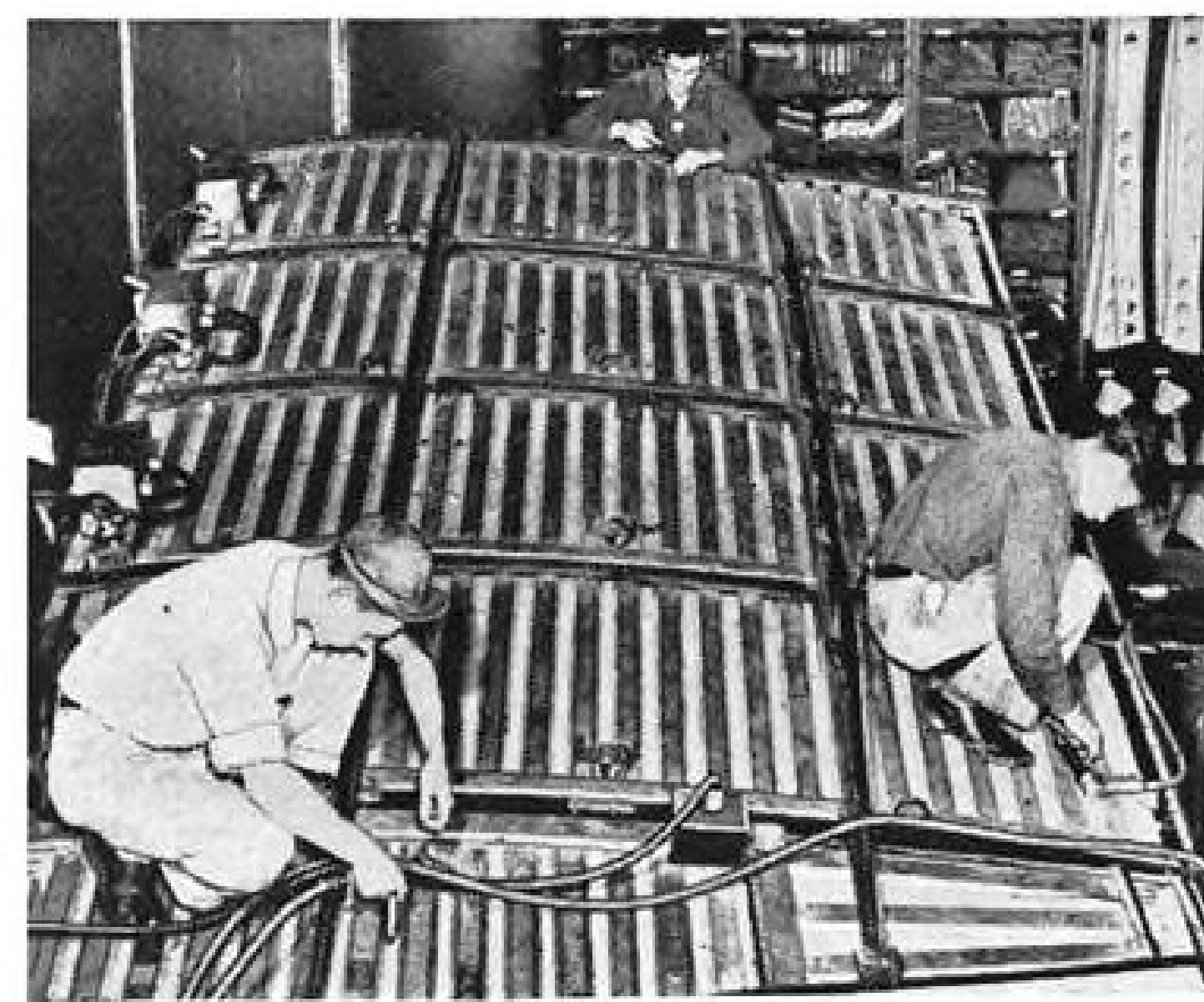
SKIN SHRINKER , ingenious product of Martin engineering, heats the aluminum skin of a plane's wing so that after riveting it cools and shrinks tightly into place without wrinkling or buckling.
