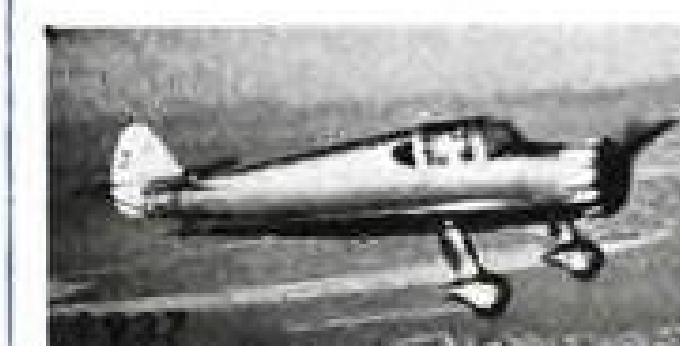
RYAN S-C, cabin plane for private-owner use, featured all-metal construction.
