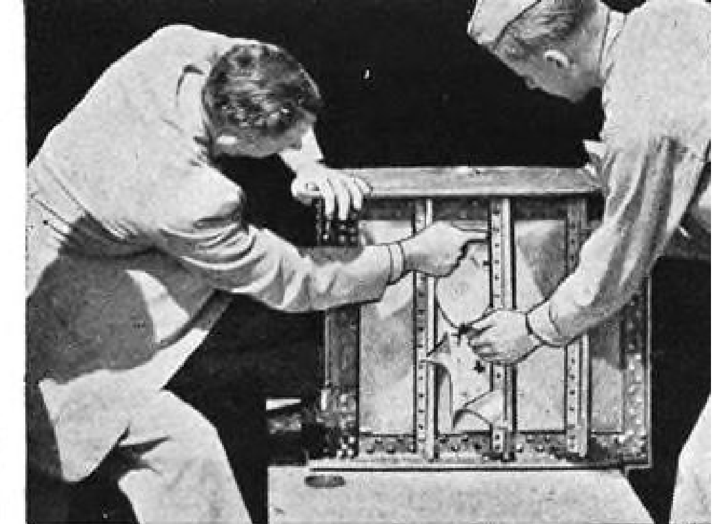
LEAK-PROOF FUEL TANKS , America's first, were developed by Martin, are now standard equipment on many makes of U. S. aircraft. Martin experiments on self-sealing fuel tanks date from 1919 in which time 285 materials were tested.
