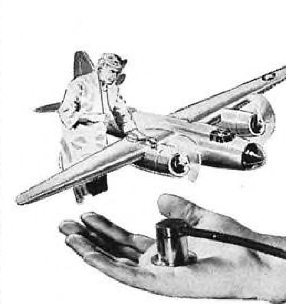
FLUTTER DETECTOR , plus accelerometer and oscillograph, enables Martin engineers to record graphically a plane's flutter characteristics. This development will aid all industry in combating vibration.
