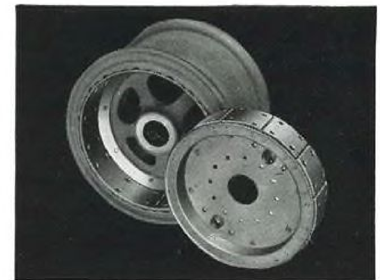
The GENERAL 9 x 12 Expander Tube Brake & Wheel—partially assembled.
