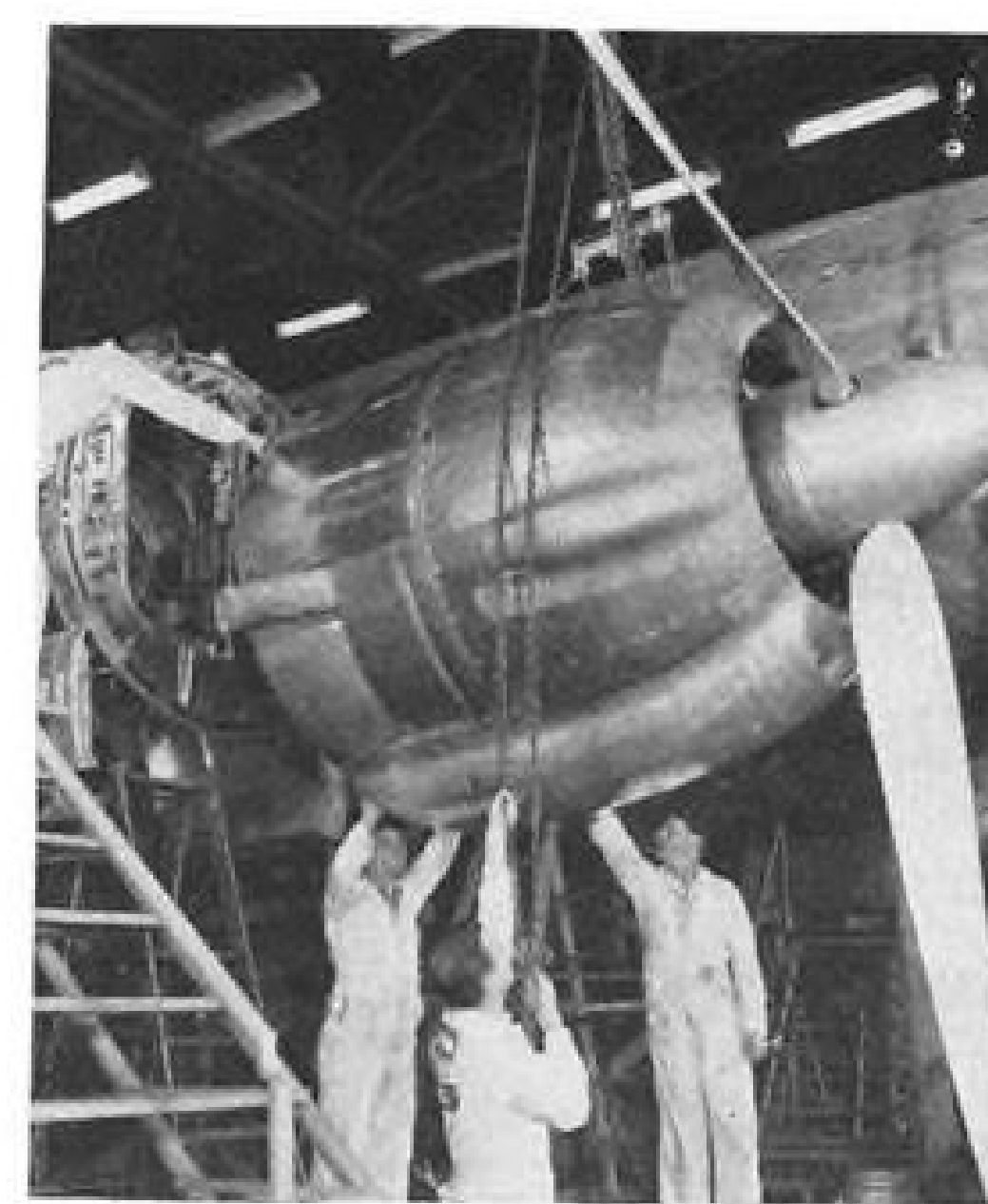
Record Power Plant Change: Lockheed engineers have developed a "power egg" system which permits a complete change of power plant in 27½ minutes, which has been applied to the new four-engined Lockheed Constellation . Photograph shows one of the steps in the quick exchange.
