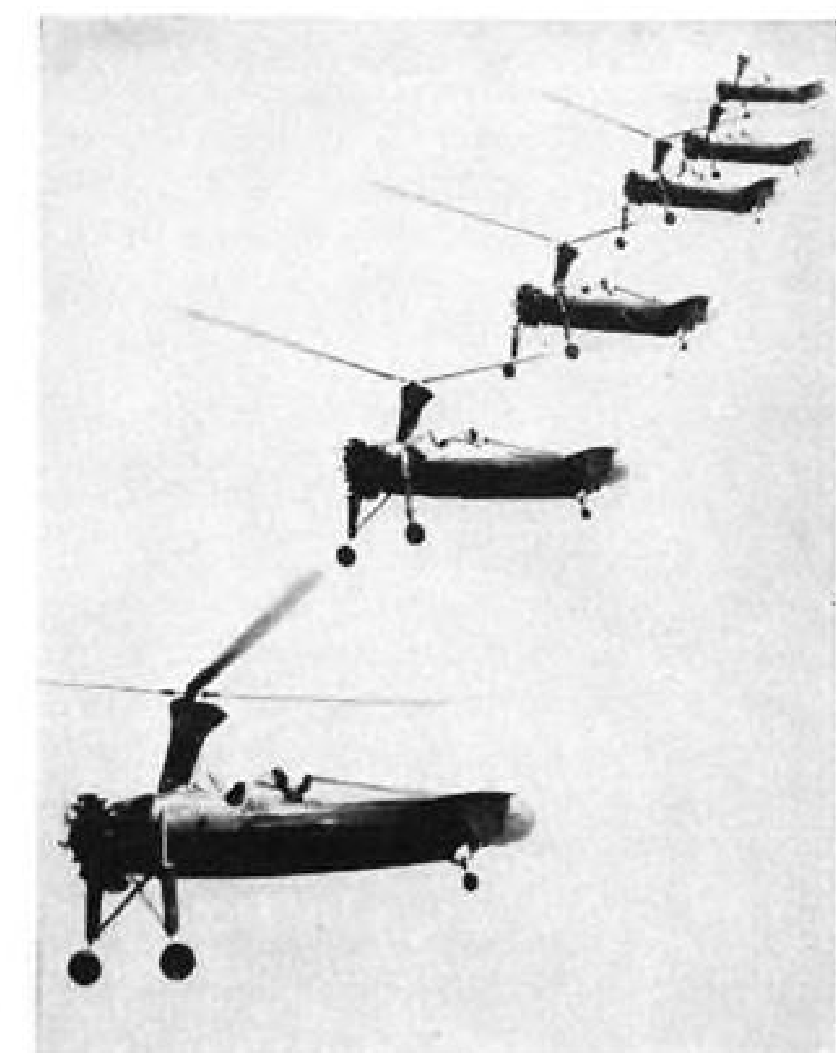
A flight of military-type Kellett rotary wing aircraft. They can land on a flat roof, plowed ground or deep grass with scarcely a turn of the wheels.
