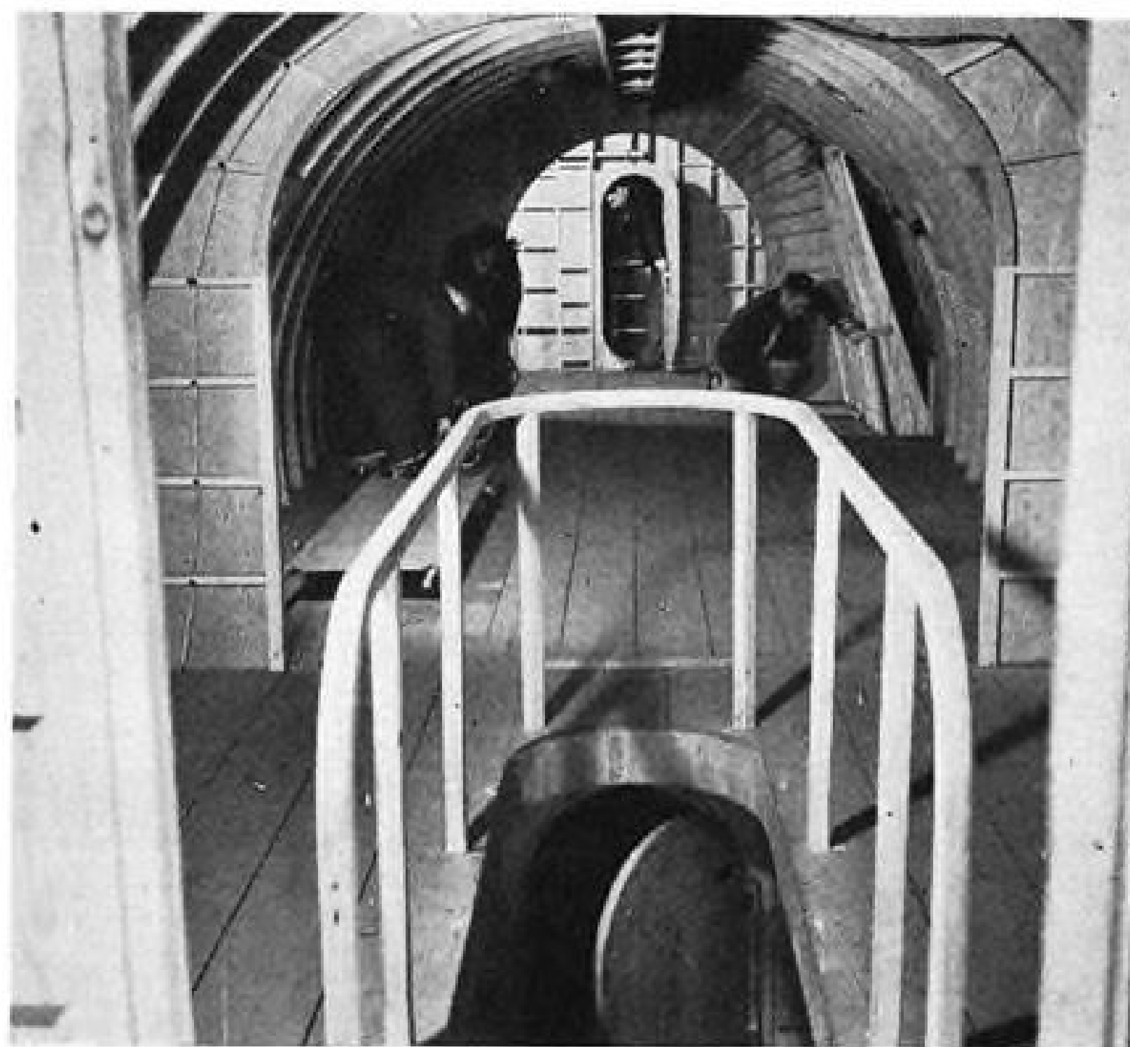
partment. Workmen above are in pilots' seats. On right, workers show how litters are handed to upper deck through special trap doors. As a hospital ship, the JRM-1 will carry 84 litter cases and 25 attendants.
