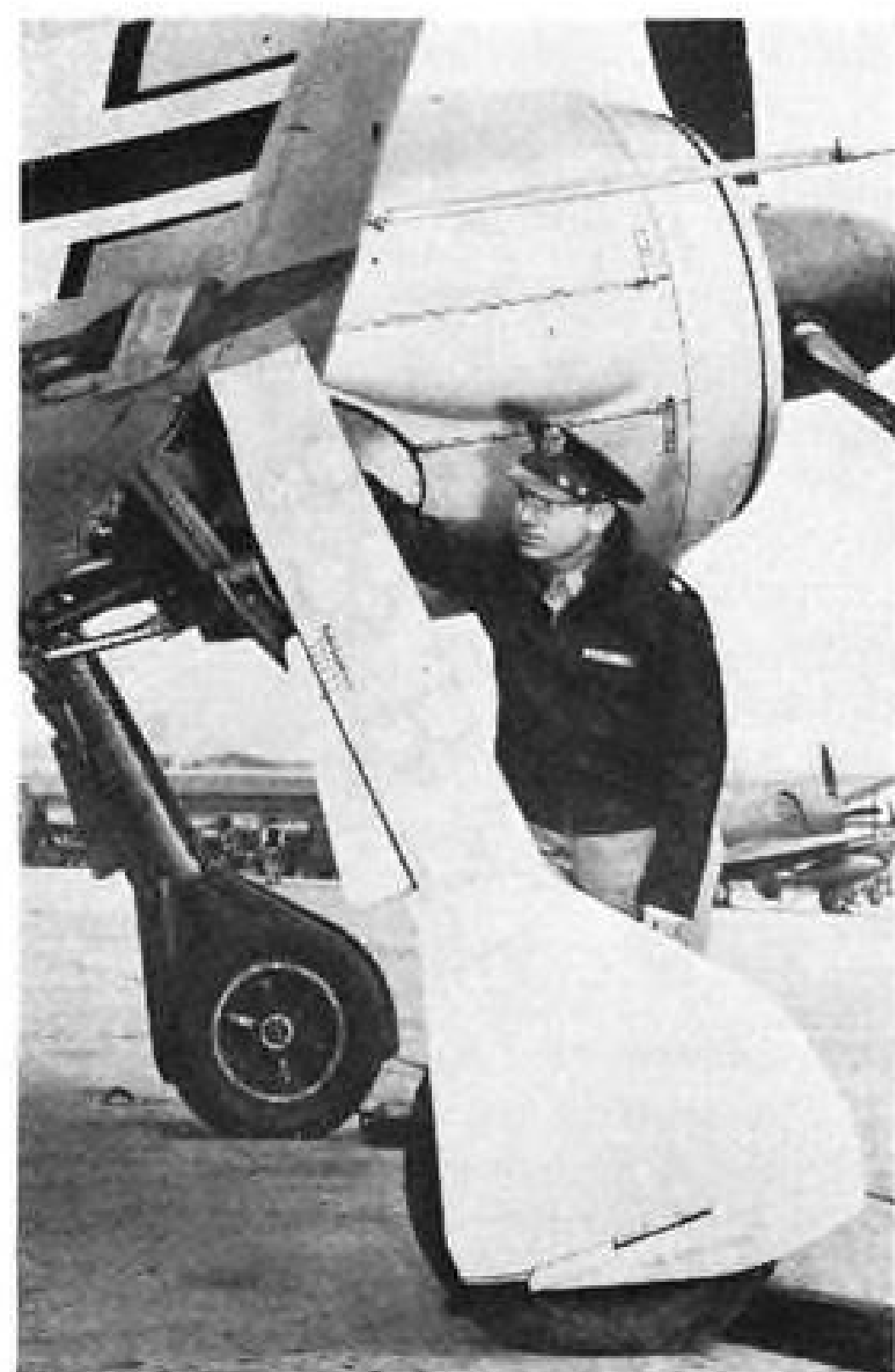
FW-190 LANDING GEAR: German type of elongated landing gear of the Focke-Wulf 109 is seen in this picture of the captured fighter now at Wright Field.
