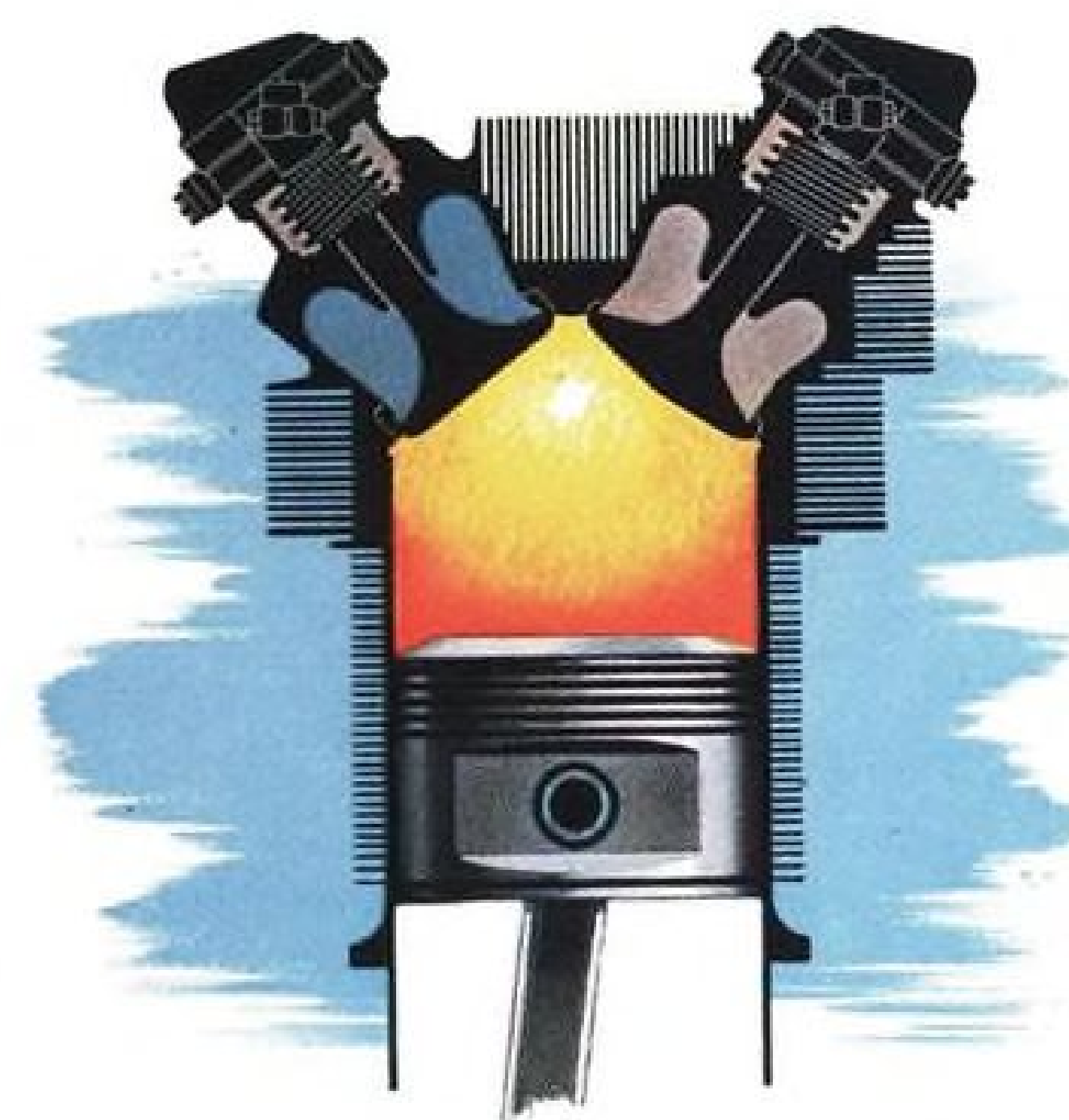
The Wright forged-head cylinder has permitted a 15% increase in power without increase in weight.
