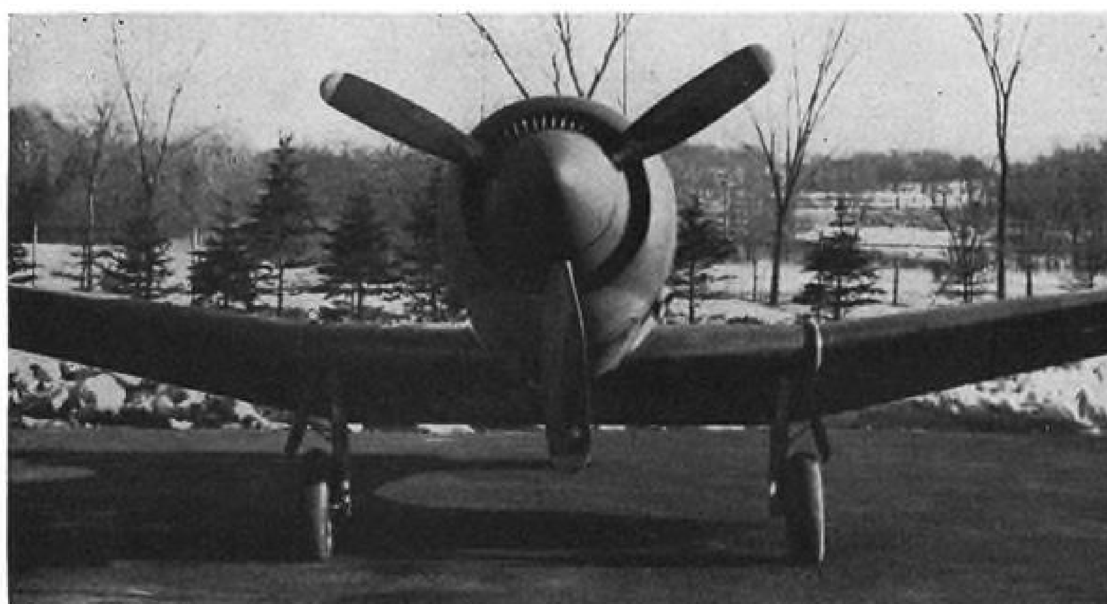
Newly Developed Engine Cooling Fan: The many-bladed fan shown mounted on the propeller shaft of a Wright Cyclone engine, and as it appears installed on a plane, has been developed by Wright Aeronautical
