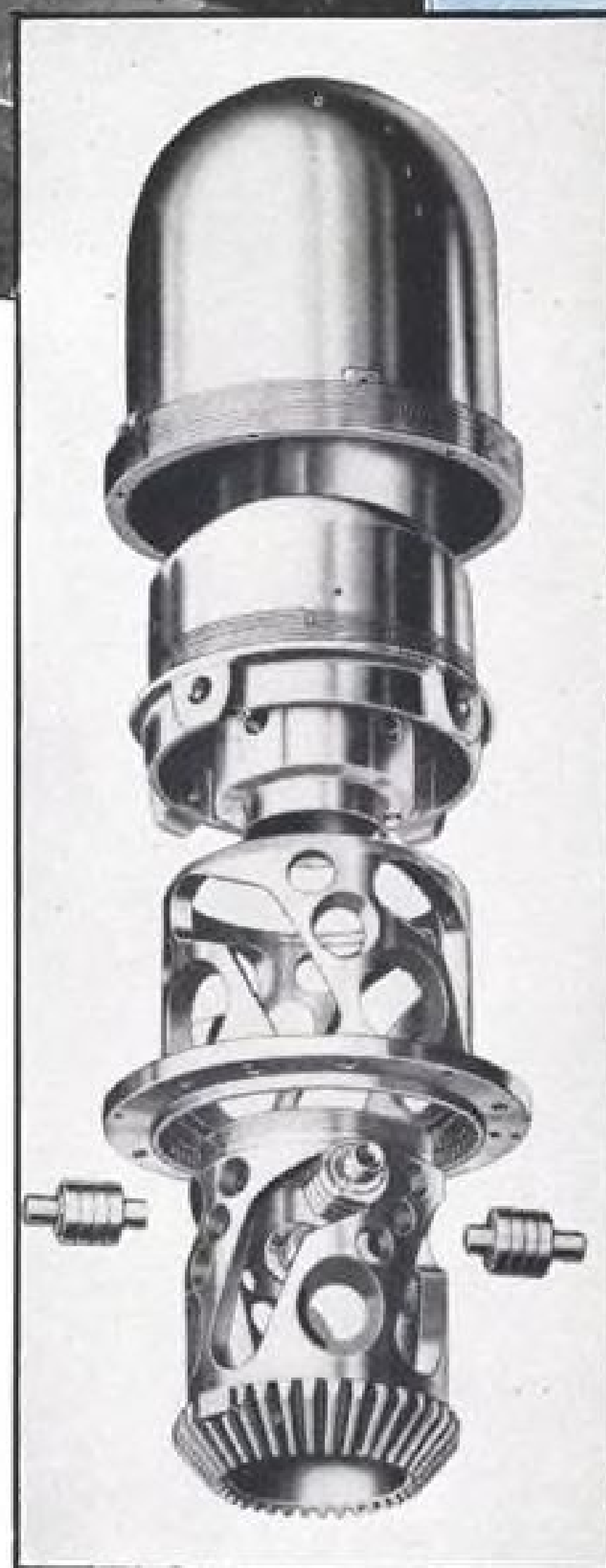
One of the greatest aids to modern aviation is the Variable Pitch Hydromatic Propeller whose barrel and cam set-up is shown above.
