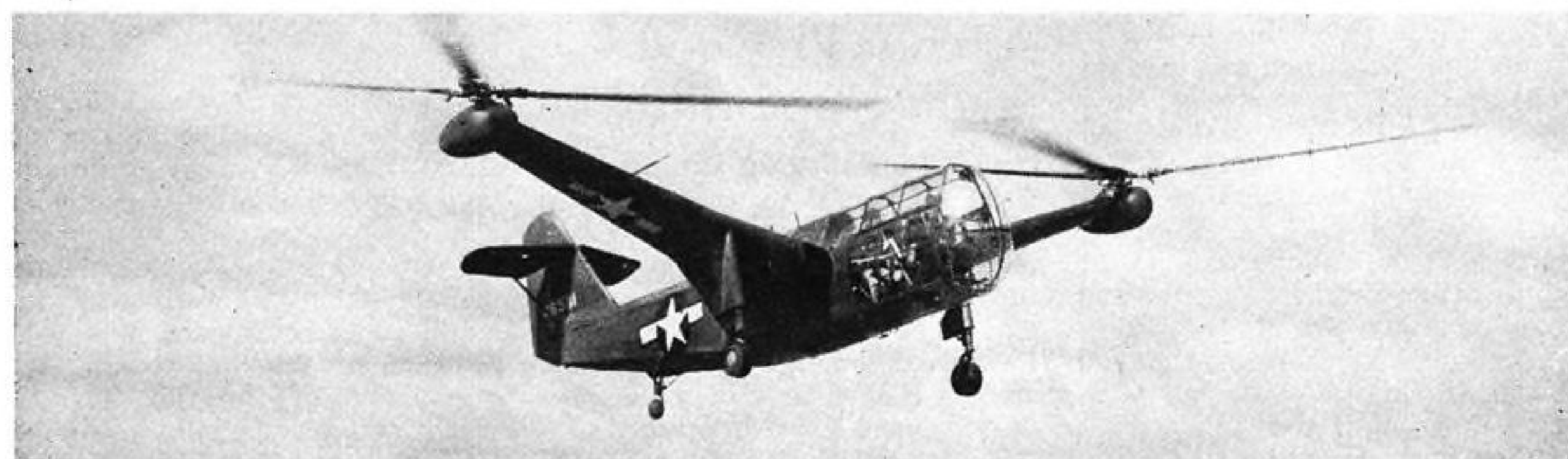
New Platt-LePage Twin-Rotor Helicopter Tested by Army: Shown is the XR-1A in hovering flight over Wright Field, AAF Materiel Command headquarters, at Dayton, Ohio. The craft follows a design basically
