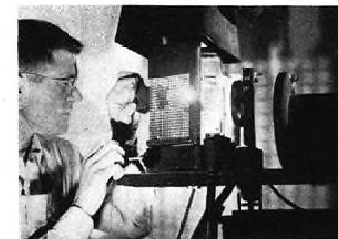
SPECTROGRAPH... Analysis determines exact characteristics of metals to be joined.
