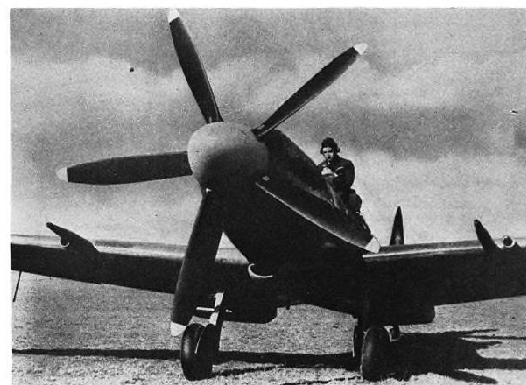
"Spitfire" XIV Disclosed In Action: Two views of the new Spitfire powered by Rolls-Royce Griffon 65 engine developing over 2,000 hp. and utilizing a five-bladed propeller for the first time on modern aircraft. Plane is heavily armed, fast and has high altitude performance at a ceiling of over 40,000 feet.
