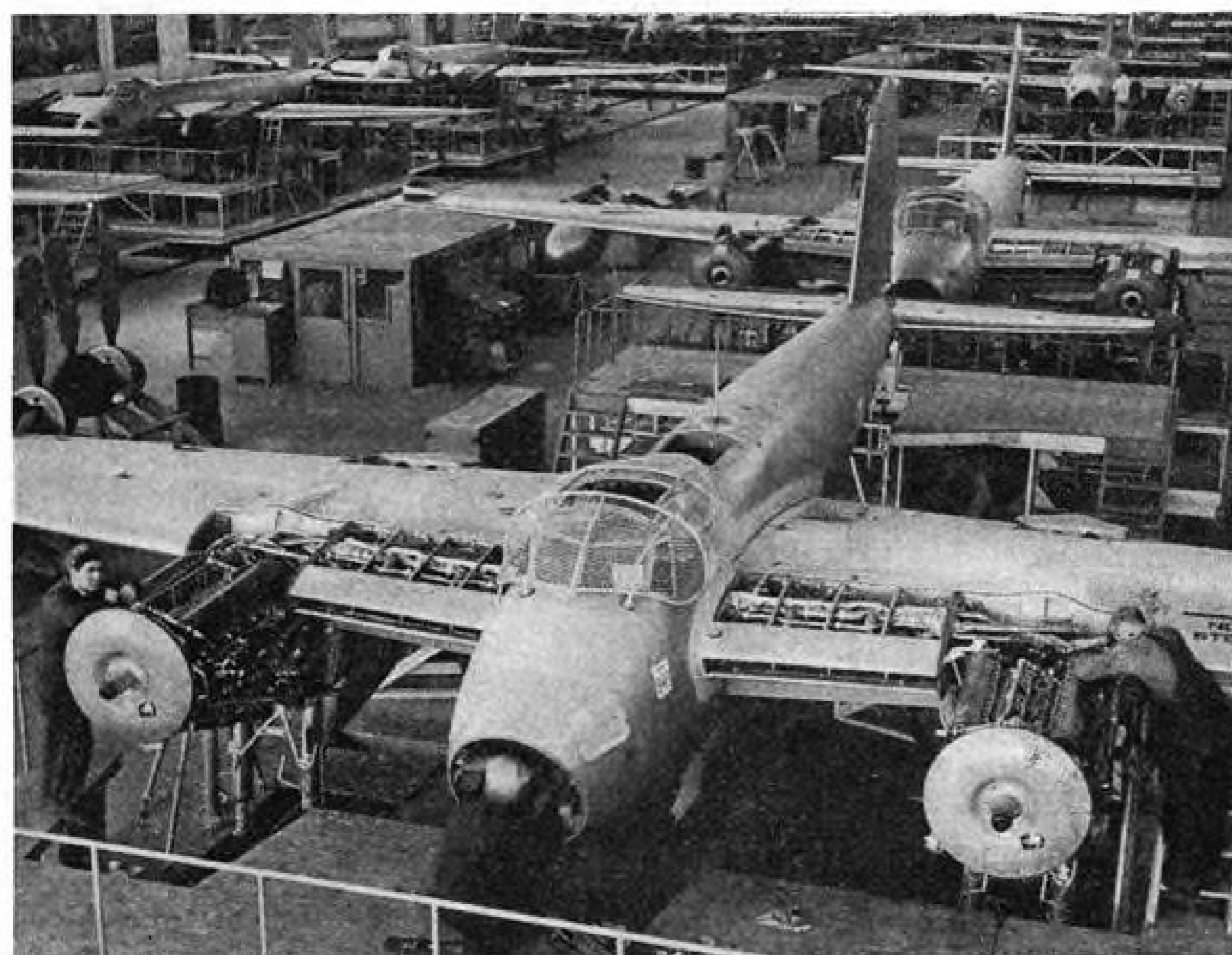
De Havilland Final Assembly Line: Final assembly bays at de Havilland Aircraft of Canada, Toronto, where Mosquito bomber-fighters are produced for Allied airmen on a moving assembly line. Wire screen cage over cockpit top protects lucite.
