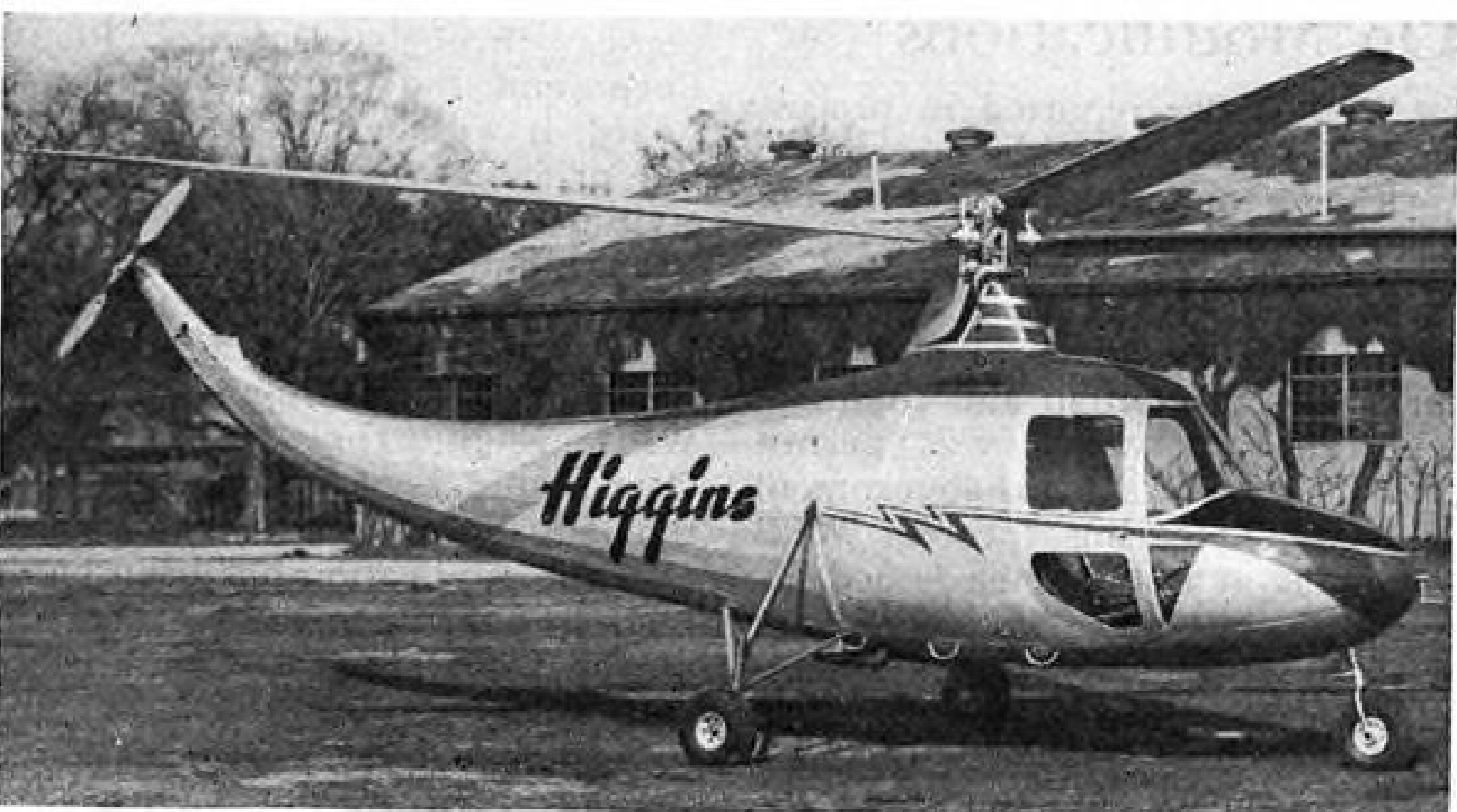
Higgins' Double See-Saw Helicopter: Stream-lined Higgins helicopter, designed by Enea Bossi, is reported to have made limited test flights, tethered with a rope, at New Orleans. Grover Loening, rotary-wing aircraft expert, described the Bossi design recently as a variation of the see-saw type, with solid rotor blades which pivot at the center.
