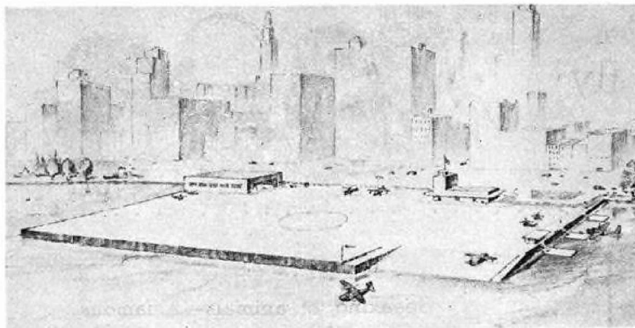
Proposed East River Sky Dock: Design of P. H. Spencer, Republic engineer, for a New York sky dock or harbor for amphibians, seaplanes and helicopters, would be built by fill-in along East River drive to provide a parking and service area for 45 to 50 aircraft.
