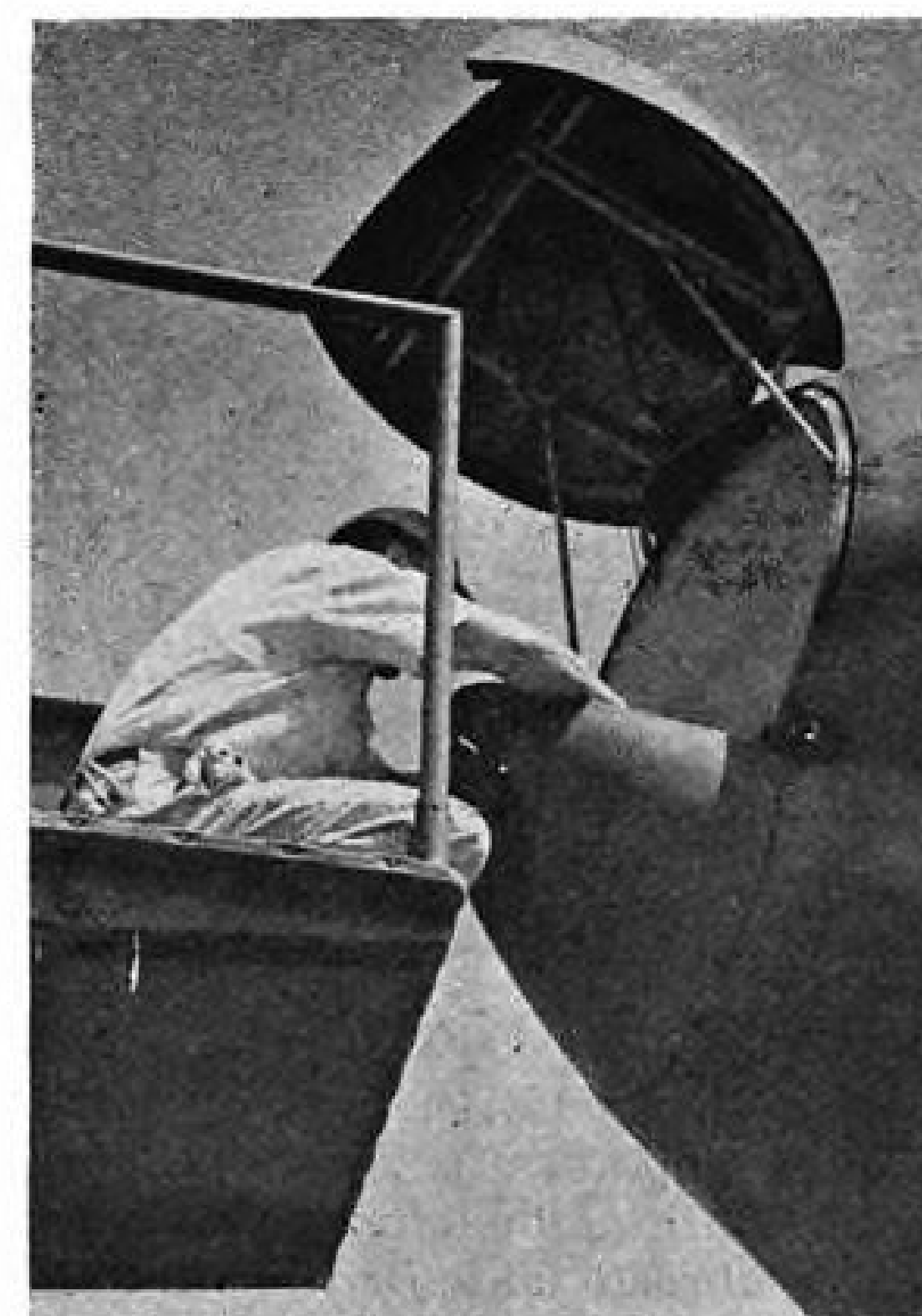
Hinged nose cone on Curtiss CW-20E gives quick access to back of instrument panel.
