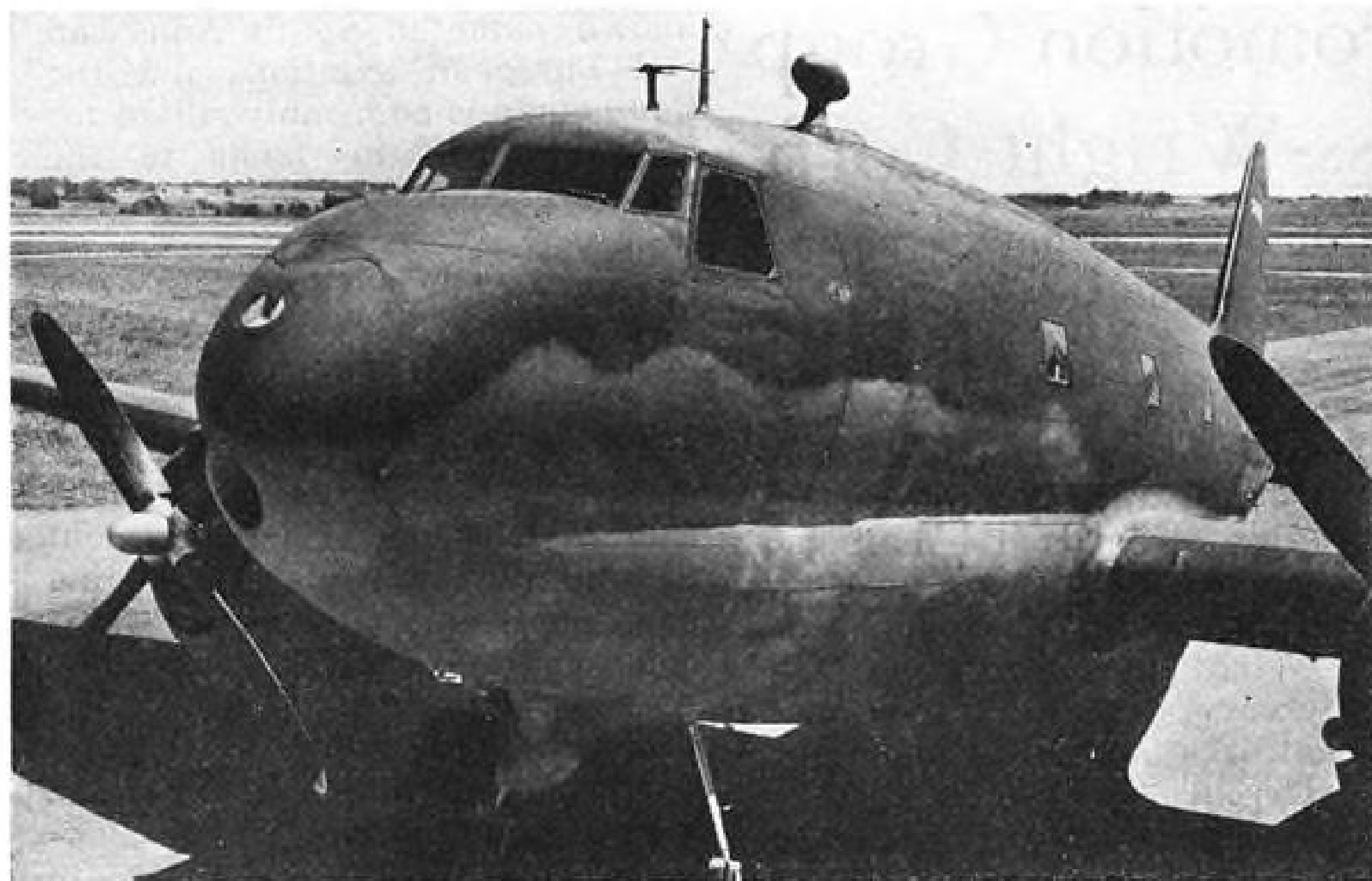
Closeup of New Recessed Nose of C-46: The familiar cigar-shape of the Curtiss-Wright C-46 Commando has been changed in favor of this new version, now going on military ships and to be a feature of the Commando airliner. The new nose gives better pilot visibility. It is "bird-proof" and equipped with a special de-icing system. The small window at the side of the windshield can be opened by the pilot without getting any air blast. The side window is a conventional slide-back type, but has a pressure-locking device for bad weather operation.
