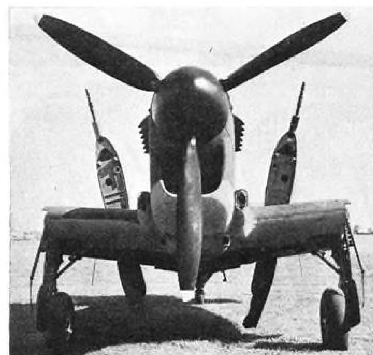
New British Naval Air Fighter for Pacific: This new already gone into service. Note the unusual folding heavily armed fighter reconnaissance plane—the wing arrangement. The Firefly is fitted with four Firefly which will operate from British carriers has 20 mm. cannon and equipped with a camera.
