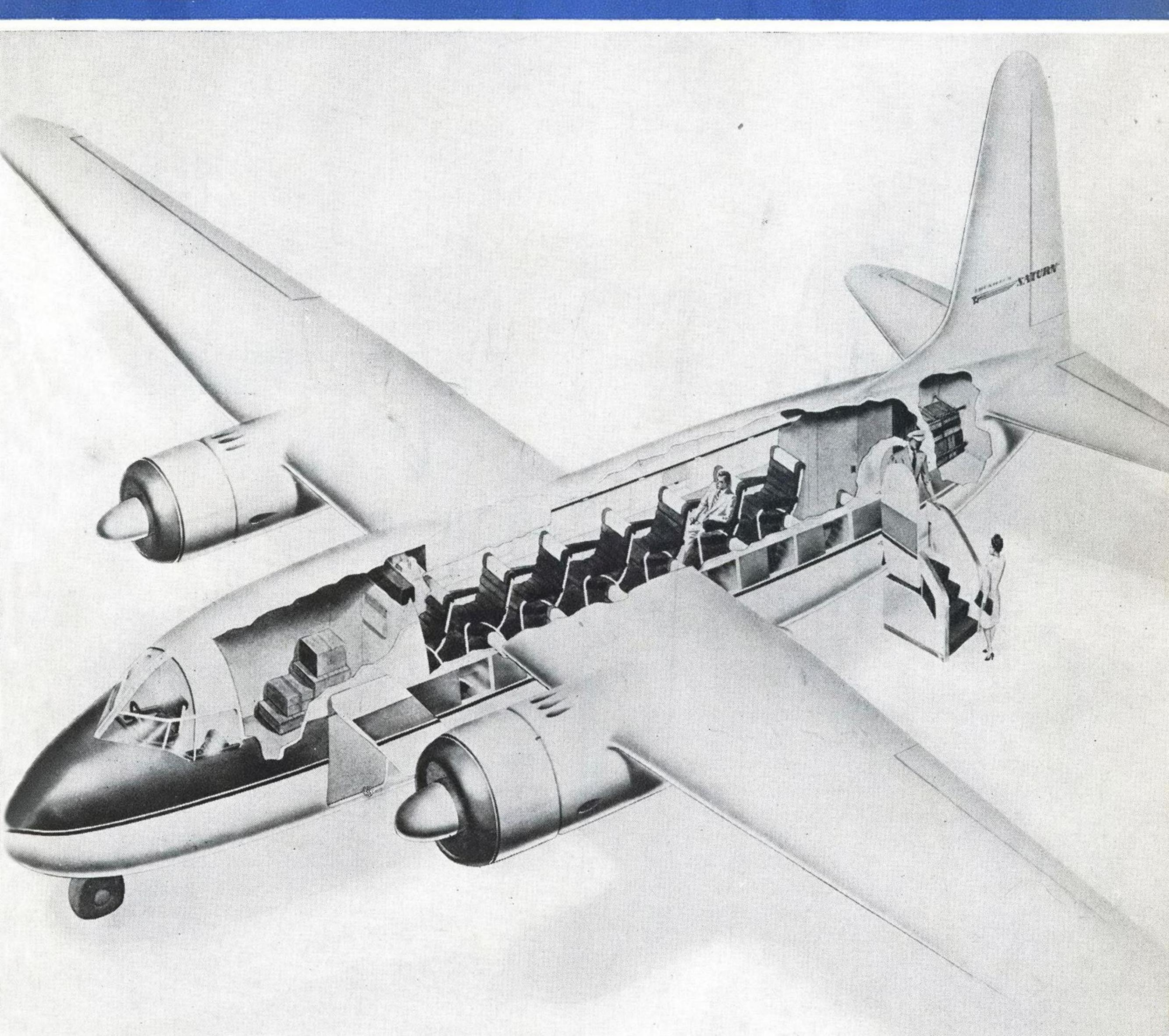
Lockheed's Post-War Saturn 75 Aimed At Feederlines: This new airplane, designed for short-haul, high-frequency airline operation, has a cruising speed of more than 200 mph., carries 14 passengers, a crew of two, baggage and cargo in the standard version.
