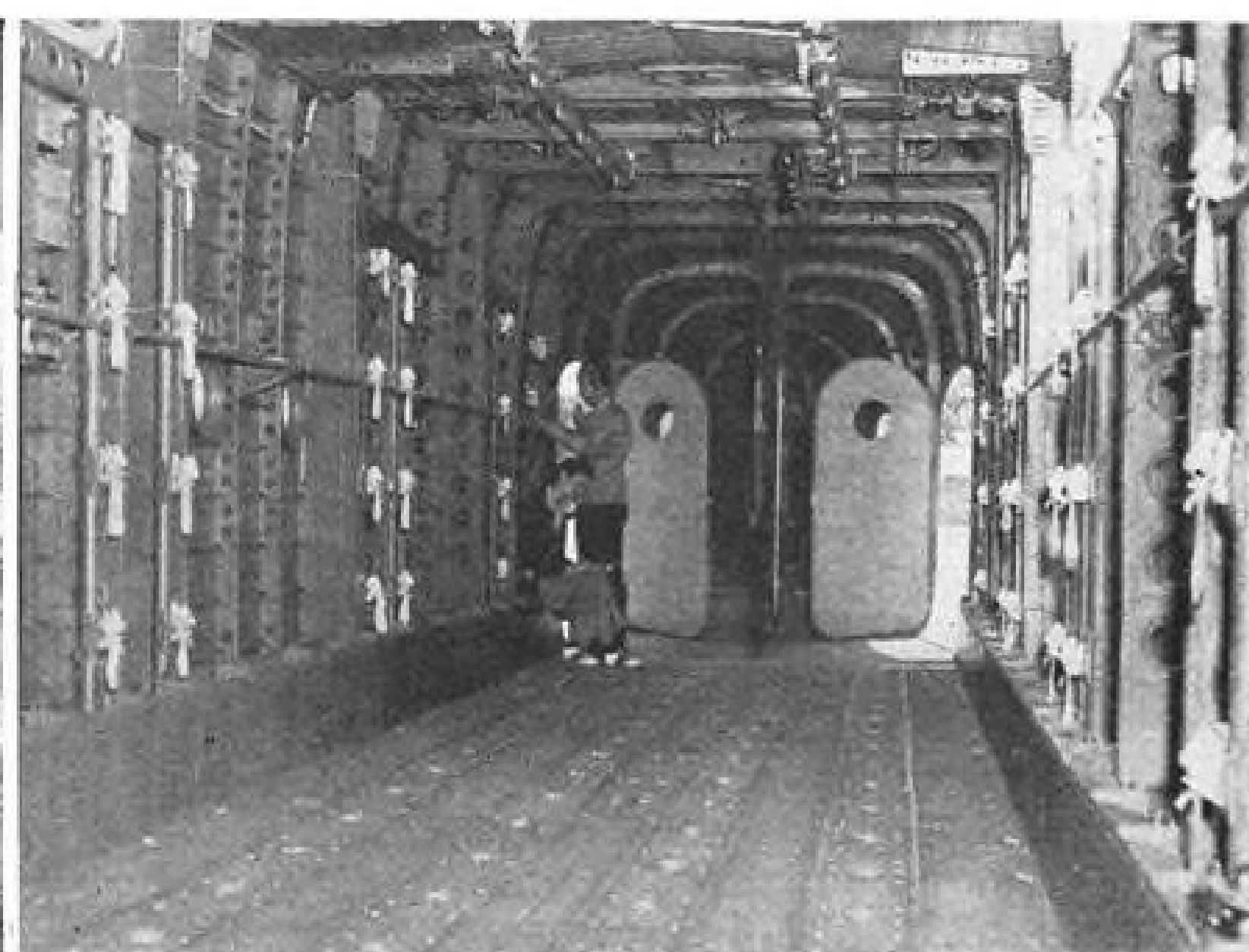
two small "jump doors" for paratroopers are cut in the double rear doors which open to full width when the ship is to be loaded or unloaded. A side loading door is at the forward end of the cargo compartment.
