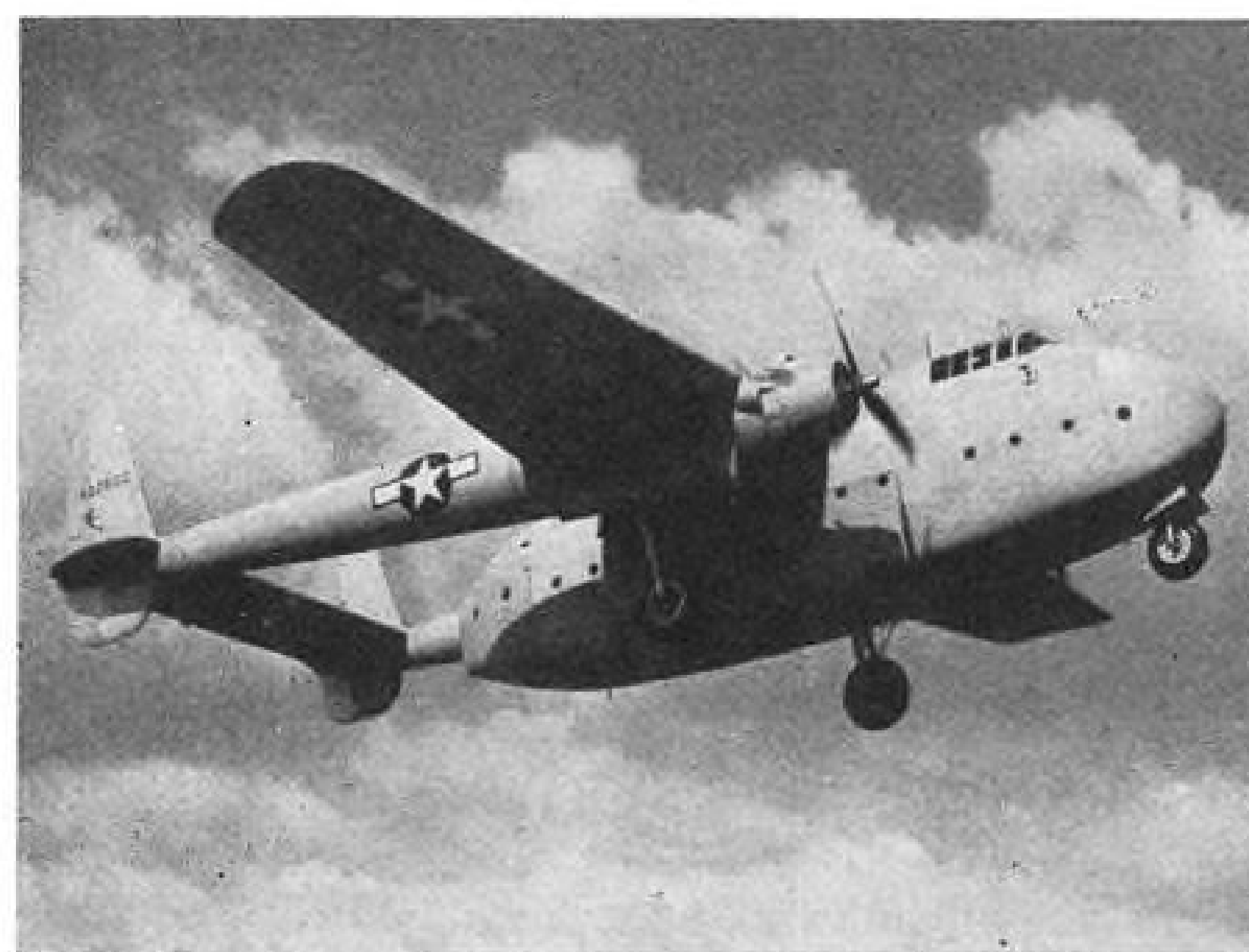
Outside and Inside the C-82: Picture of the C-82 Packet in flight shows how the box-like fuselage is carried between the twin booms. Interior view, looking towards rear, shows square construction. The
