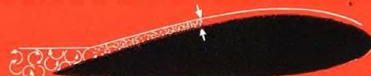
This diagram illustrates how turbulence is reduced when roughness of surface is eliminated by use of Laminar Flow Screws.
