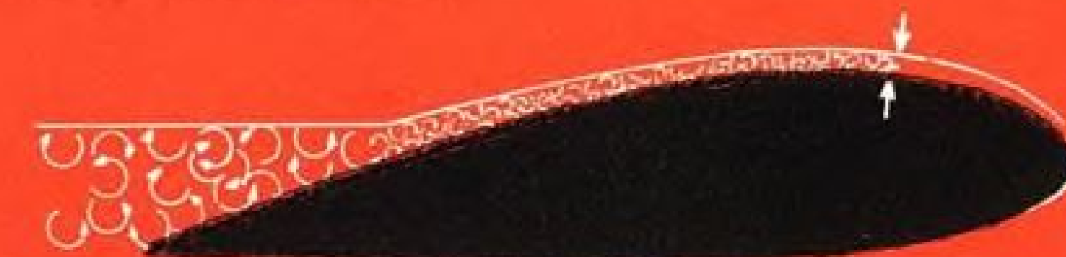
Diagram above illustrates effect on air flow on upper surface of air foil when turbulence is caused by lack of flushness of screw heads.
