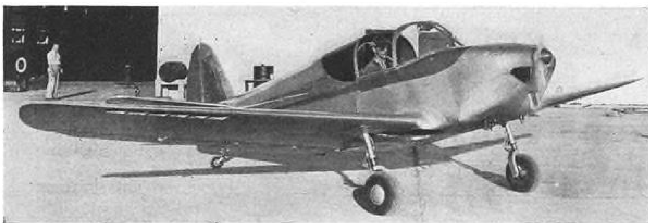
"Swift" Revs Up: Newest photo of the two-place Globe Swift prototype shows the plane revving up in preparation for takeoff. Wing-slots, hydraulic retractable landing gear, and sliding cockpit enclosure are shown clearly.
