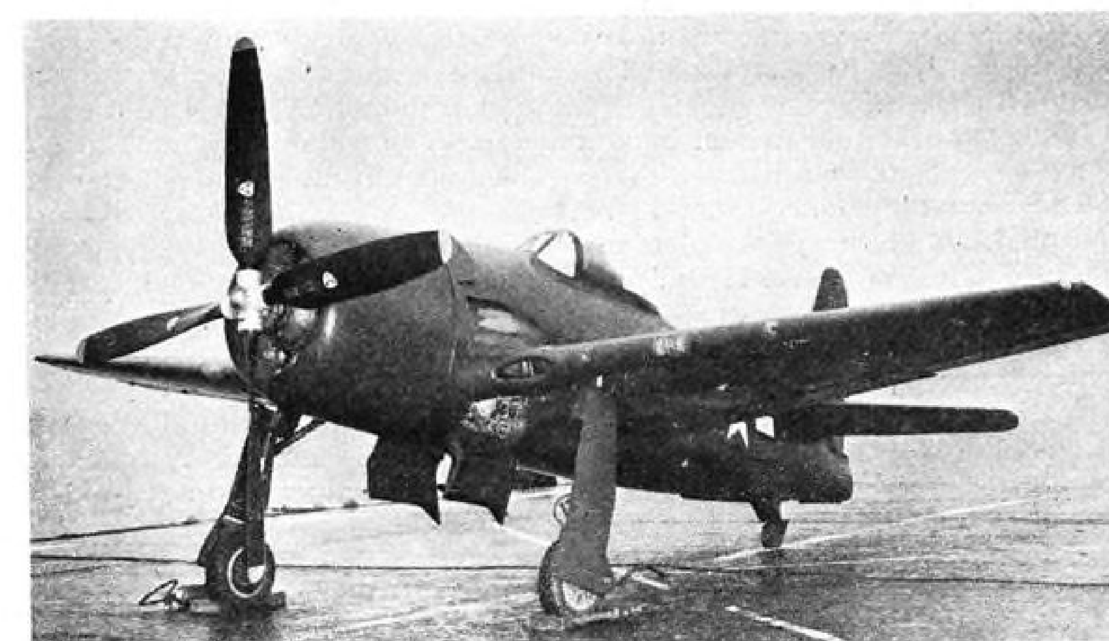
New Views of F8F “Bearcat”: This lightweight, high powered fighter, built by Grumman for the Navy, is smaller than its close kin, the Hellcat and Wildcat. Consequent lower drag makes it possible to put more aboard carriers, and the high horsepower makes it possible for them to take off with almost zero wind coming over the flight deck. The nearly 20 knot wind needed by most shipboard fighters has been a handicap to escort carriers.
