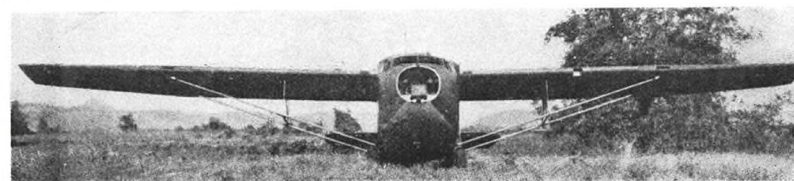
The Mitsubishi Ku 8 Japanese military glider is shown in this photograph from The Aeroplane. Known also as the Goose, it has a wing span of 72-ft. and carries about 15 troops.
