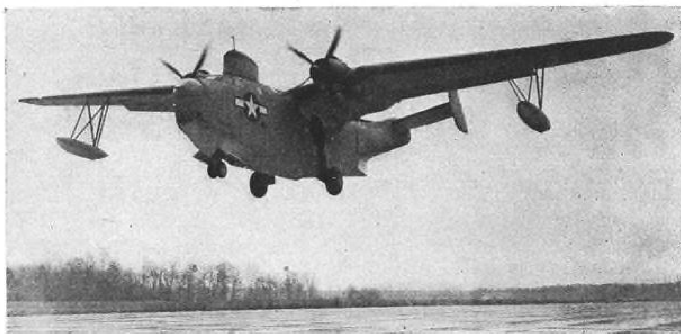
First Flight: Largest amphibian ever built, the Martin XPBM-5A takes off on its first test hop from the company field at Middle River, Md. The ship is a modification of the Mariner, gull-winged flying boat widely used by the Navy.
