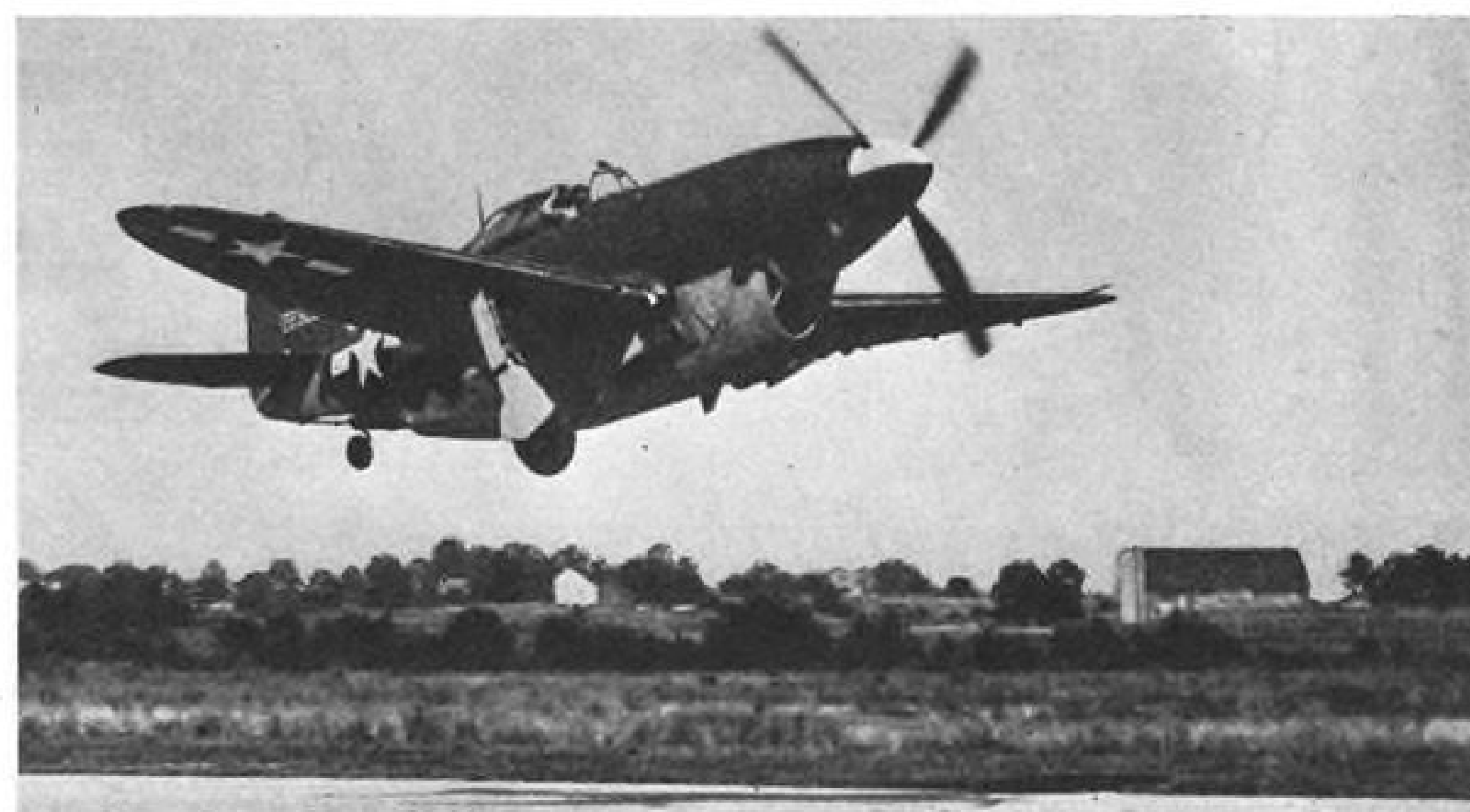
Novel "Thunderbolt": This tapered-nose P-47 was specially rebuilt to test 2,500 hp. liquid-cooled Chrysler engine. Small frontal area of the engine made possible sleeker lines, better visibility for the pilot.
