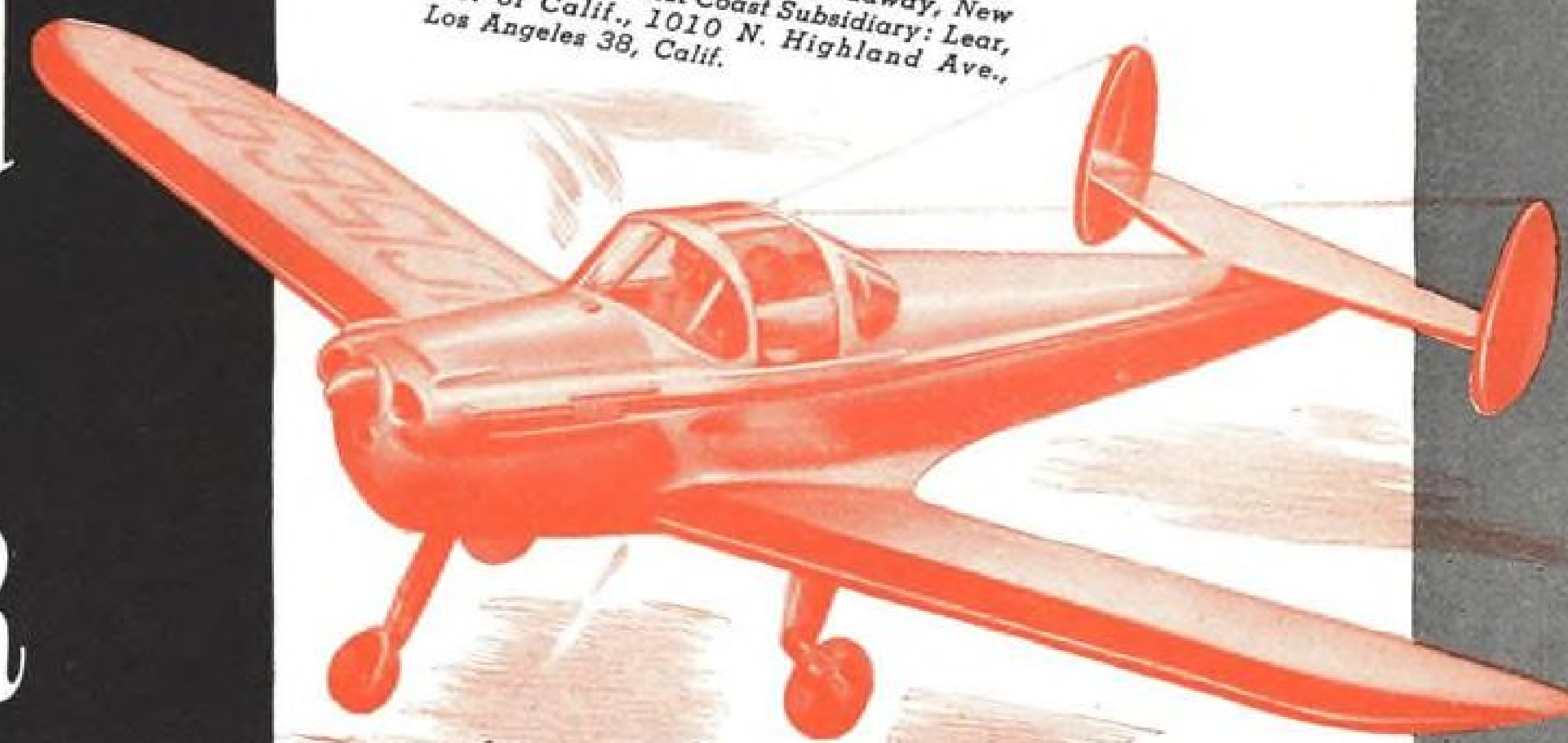
Ercoupe—compact, easy to control, all-metal light-plane—certified spinproof.
