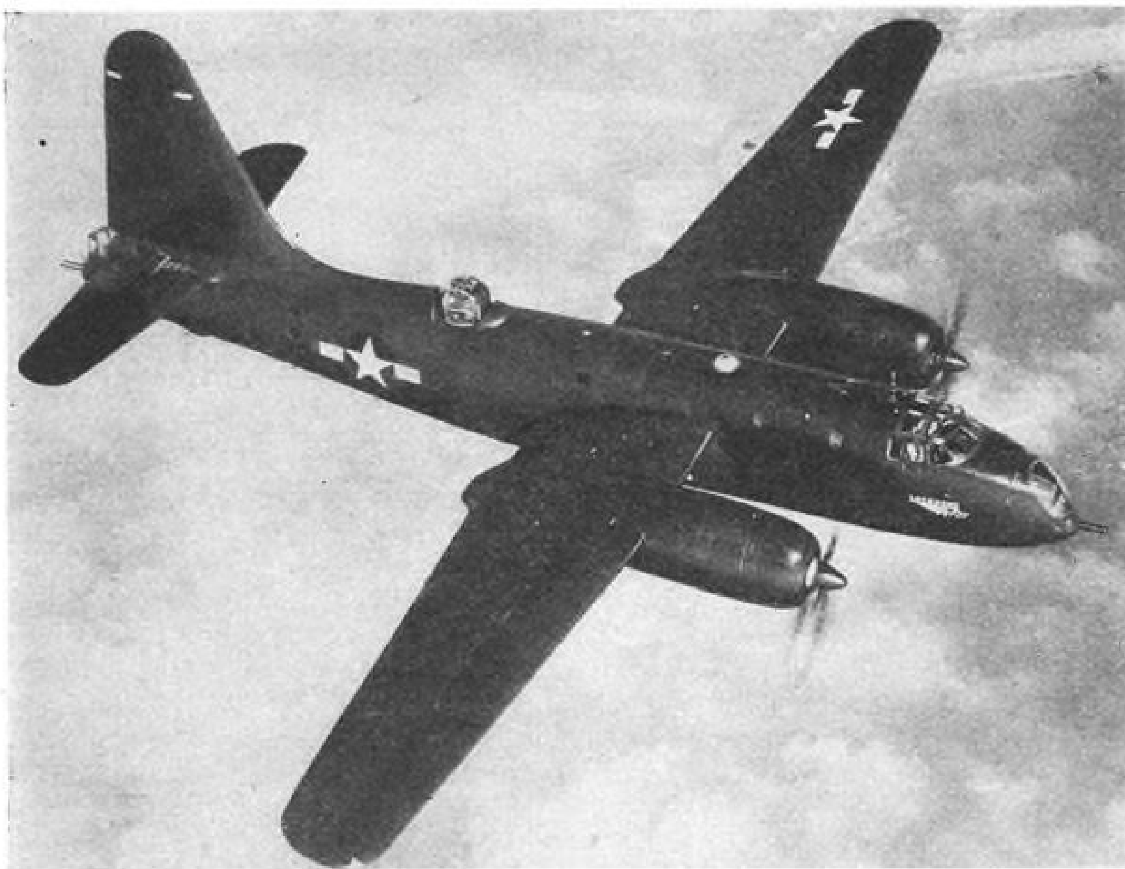
Designed for Peace: The Navy's new search and patrol plane built by Lockheed. Its range is more than 5,000 miles, its speed in excess of 300 mph. It is powered with Wright engines.
