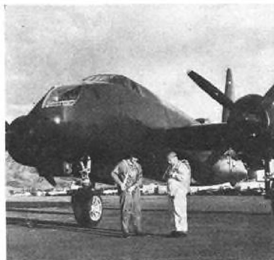
Designed for Peace: The Navy's new search and patrol plane built by Lockheed. Its range is more than 5,000 miles, its speed in excess of 300 mph. It is powered with Wright engines.
