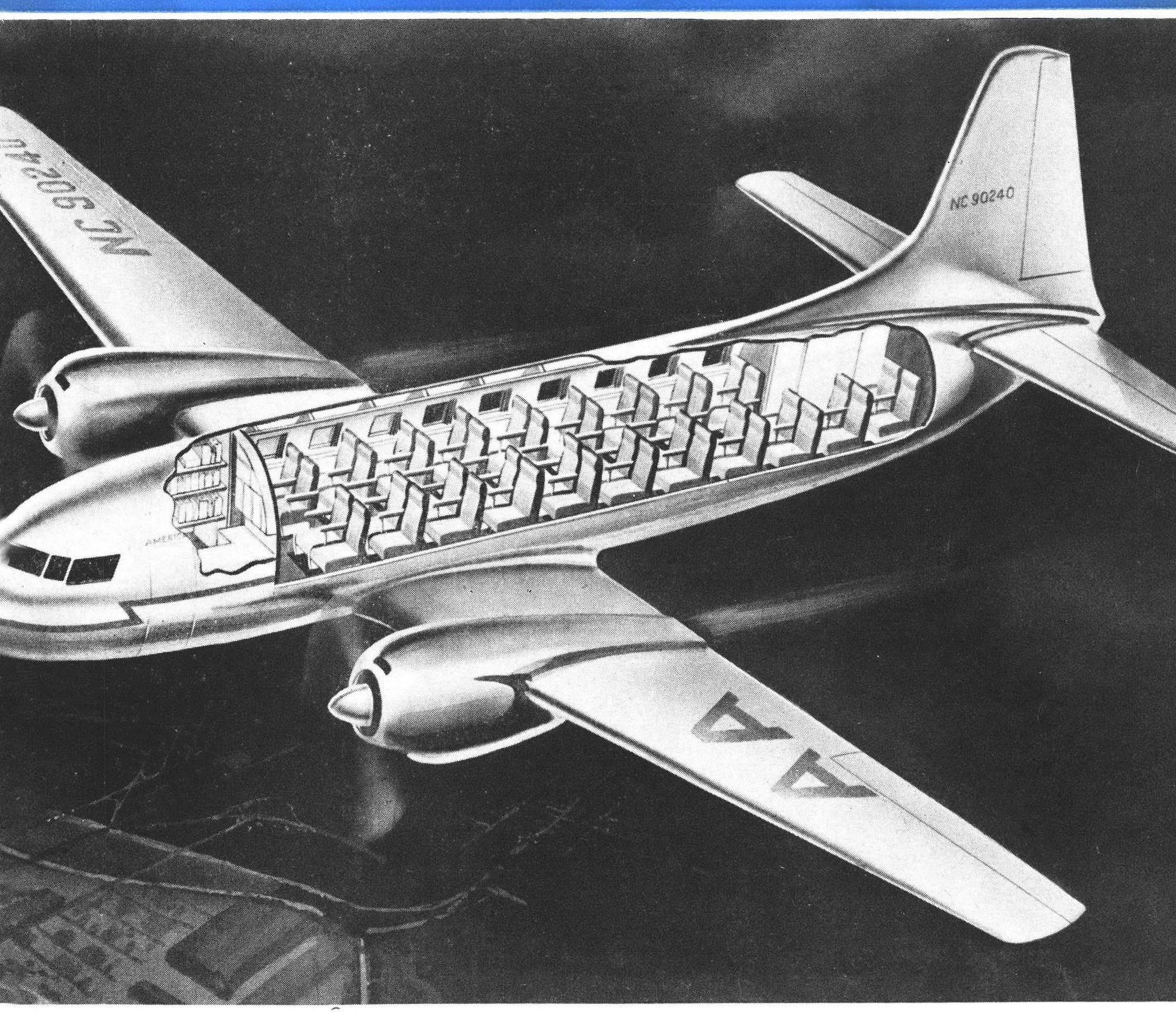
Convair's New Transport: Cutaway drawing of Consolidated Vultee's new Model 240, of which American Airlines has ordered 100 to cost \$18,000,000, shows 40-passenger seating arrangement. Using jet thrust from the exhaust of its two Pratt & Whitney R-2800's, the ship will cruise at 300 mph. and have a maximum speed of 350 mph. or above. Delivery is expected to start early in 1947. The planes will be used for flights up to 1,000 miles. (See Transport)
