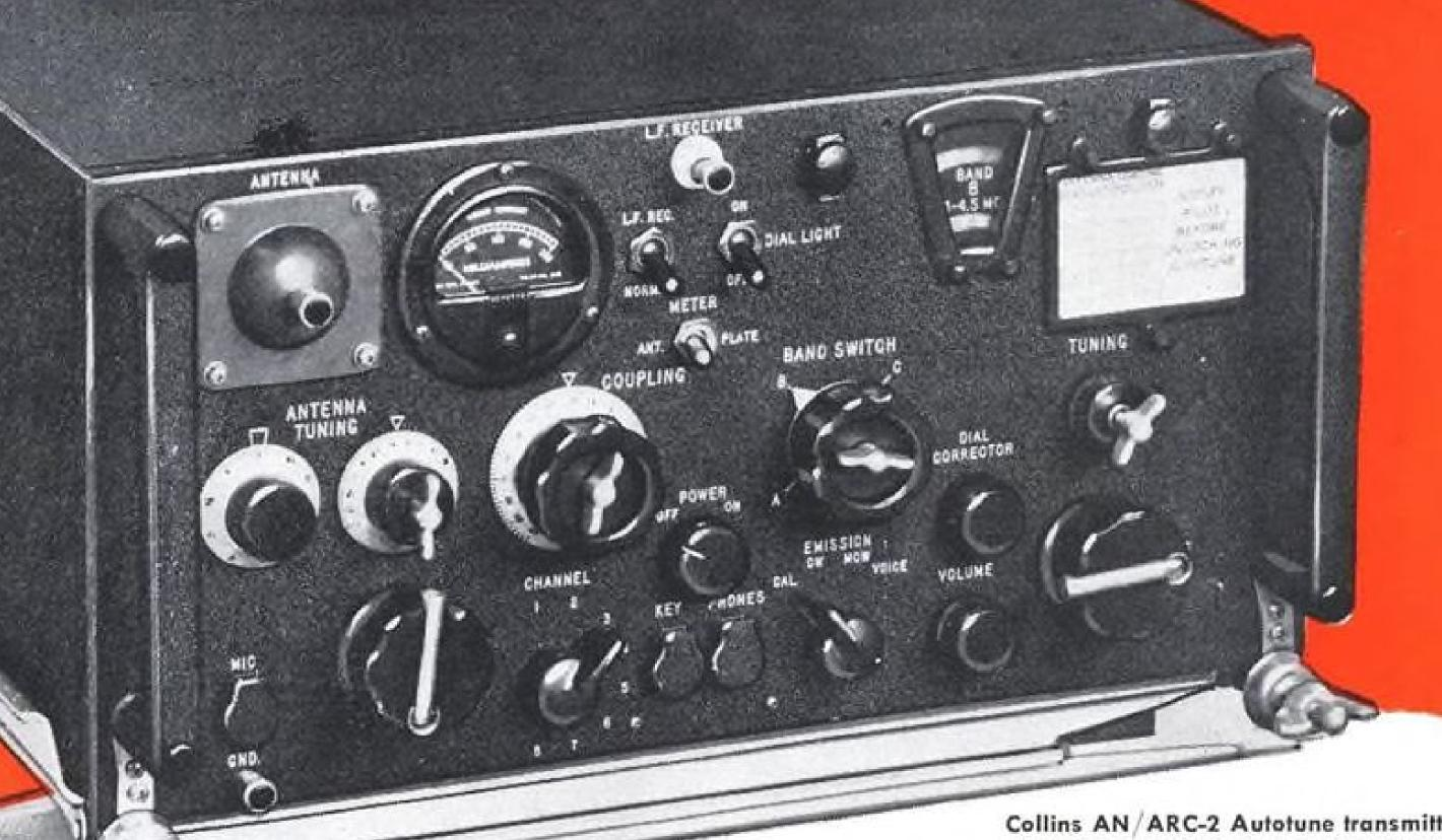
Collins AN ARC-2 Autotune transmitter-receiver
