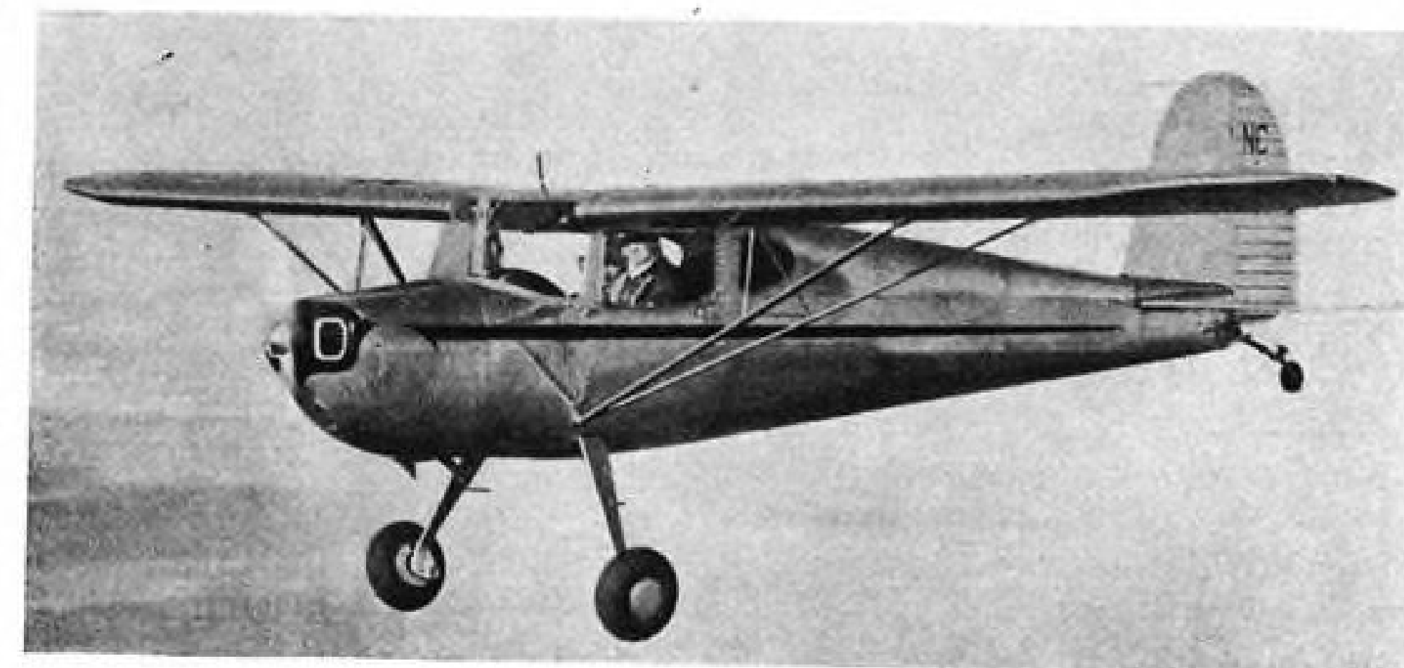
New Cessna: First photos of the new Cessna Model 120 show the new spring-steel landing gear. Despite its fragile appearance, the company reports it has withstood 20-ft. drop tests.
