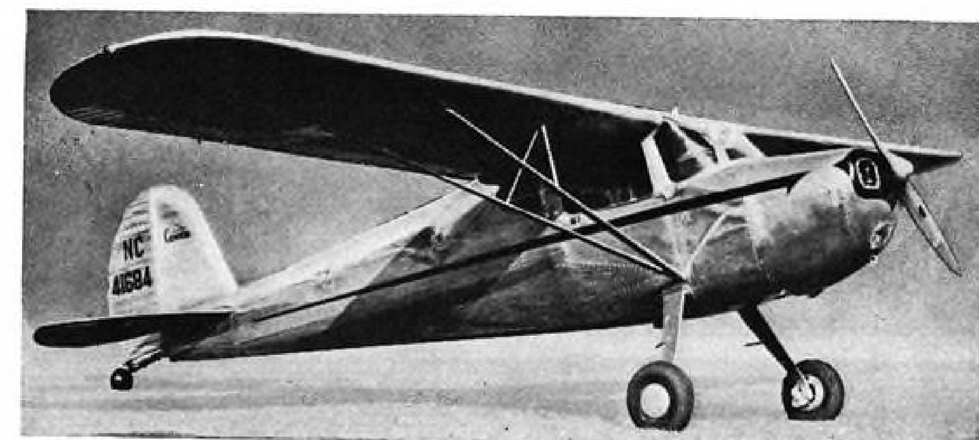
New Cessna: First photos of the new Cessna Model 120 show the new spring-steel landing gear. Despite its fragile appearance, the company reports it has withstood 20-ft. drop tests.
