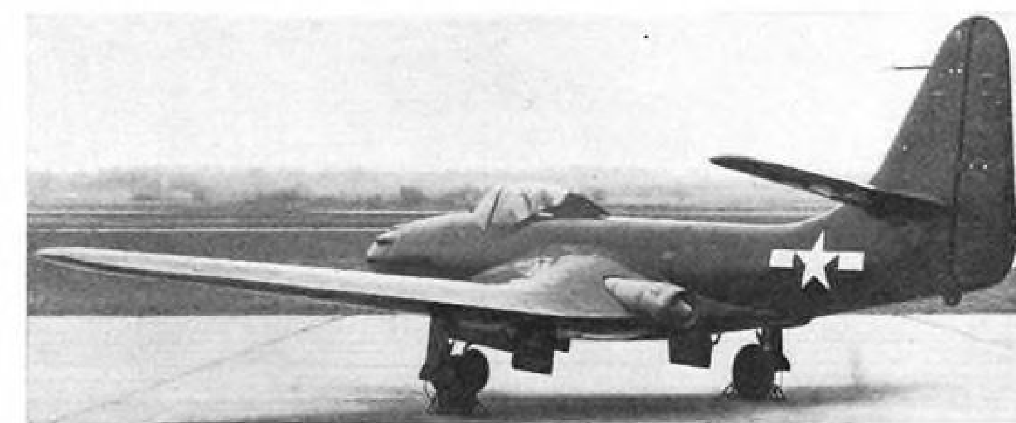
Navy Jet Fighter: Twin Westinghouse turbo-jets power this FD-1 Phantom, built for the Navy by McDonnell Aircraft Corp. Constructed of aluminum alloy, it weighs less than 10,000 lbs. with full combat load.
