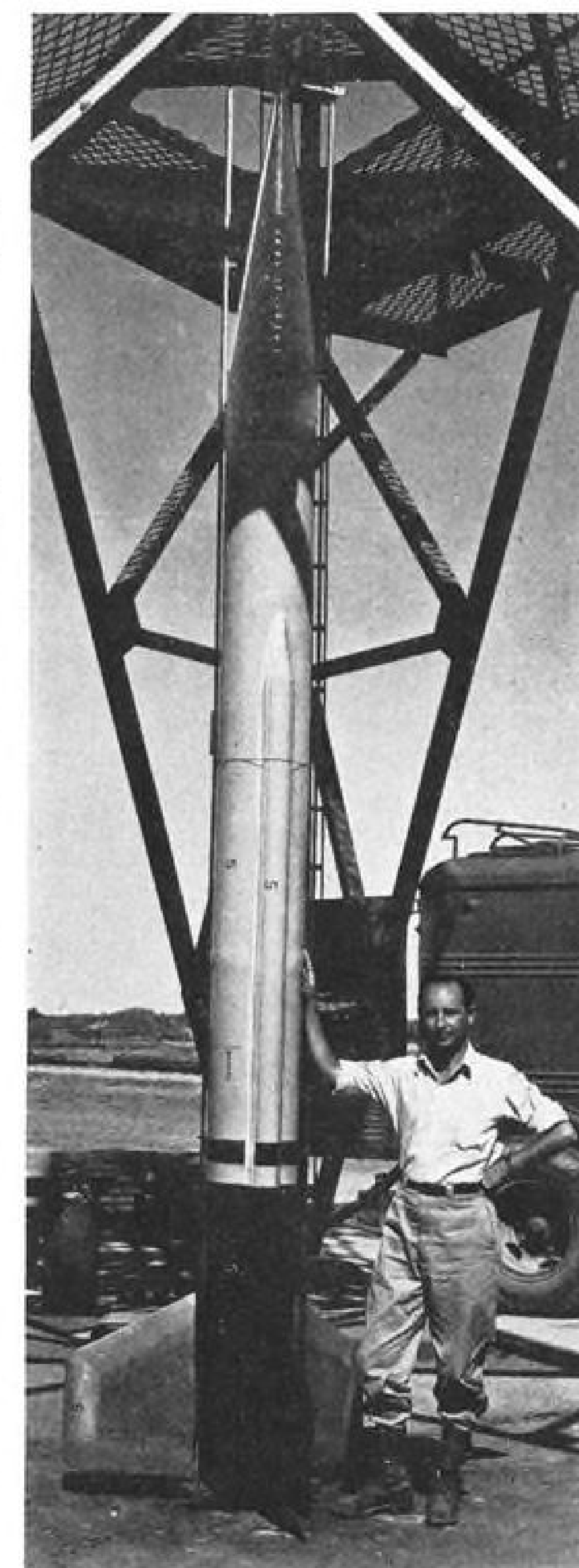
In Firing Position: A "WAC Corporal" rocket shown ready for flight in a firing tower. Standing beside the rocket is Dr. Frank J. Malina, technical director of the project and acting director of the Caltech Jet Propulsion Laboratory. The yellow center section contains the rocket's propellants. (Another photo on Page 3.)
