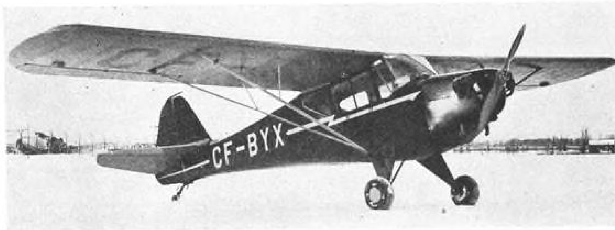
Canadian Lightplane: The Noranda, tandem aircraft being built by Noury Aircraft Ltd., Stoney Creek, Ont., for personal or instruction use.
