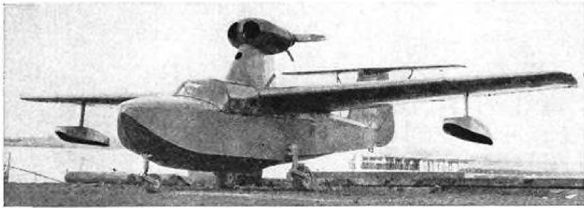
Designer and Plane: Kenneth L. Bunyard, Long Island City, designer of the Bunyard BA-X3 Sportsman, below, opens the plexiglas cockpit canopy on his three-place amphibian, a likely new entry in the personal plane field. The Sportsman has retractable tricycle landing gear, trim plywood hull, and neatly faired engine mount.
