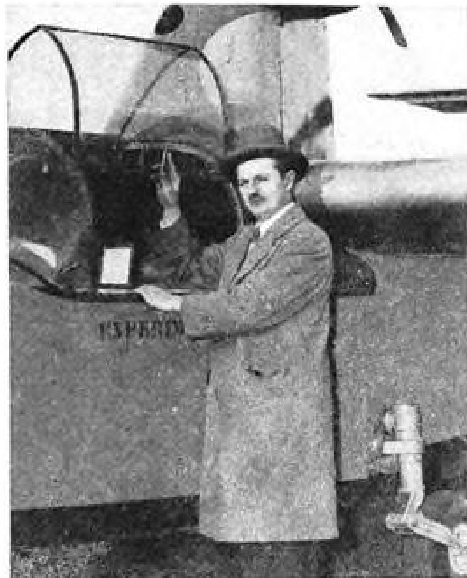
Designer and Plane: Kenneth L. Bunyard, Long Island City, designer of the Bunyard BA-X3 Sportsman, below, opens the plexiglas cockpit canopy on his three-place amphibian, a likely new entry in the personal plane field. The Sportsman has retractable tricycle landing gear, trim plywood hull, and neatly faired engine mount.
