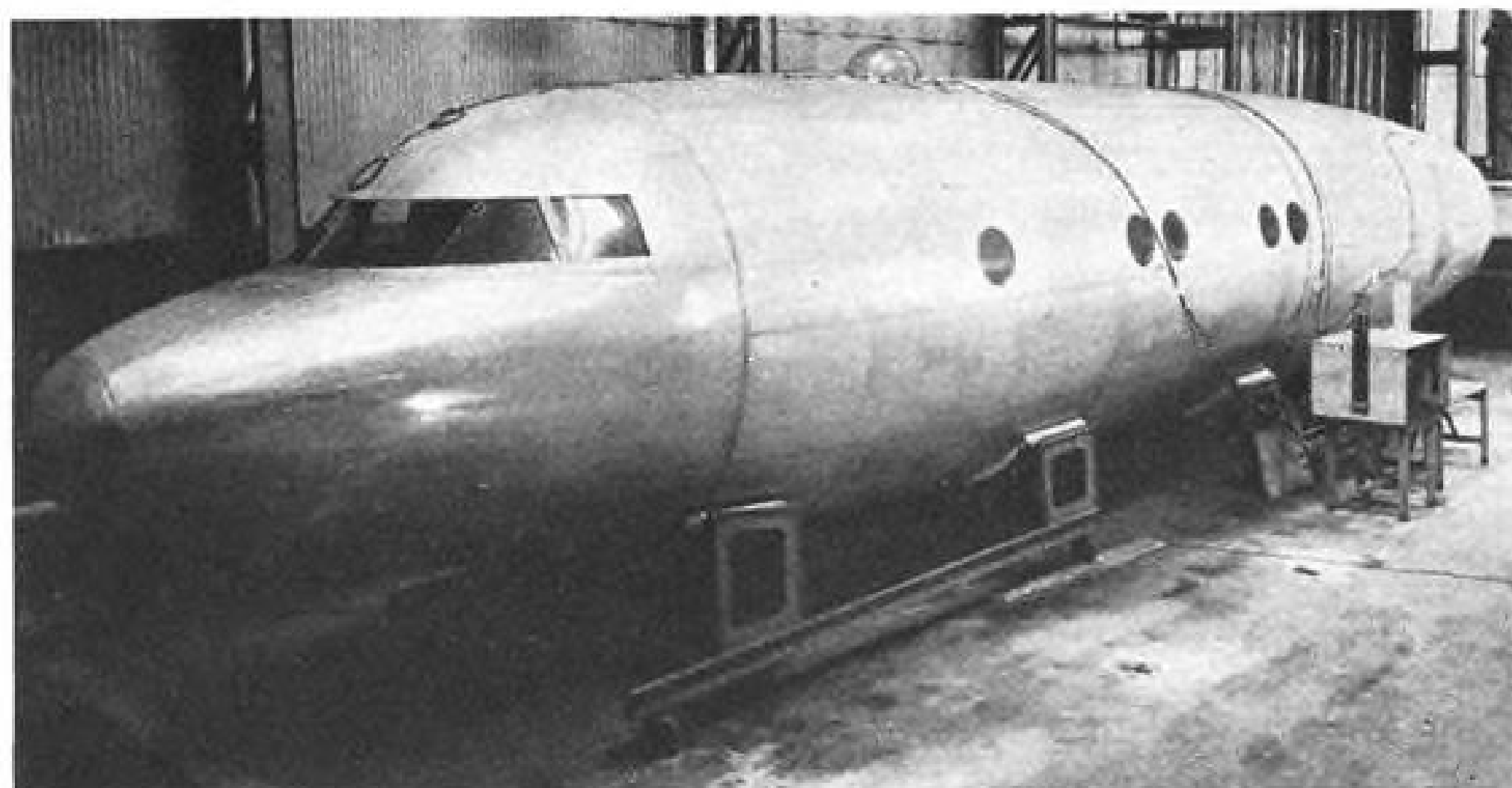
Pressure Tests on "Tudor I": Full size test fuselage of the Avro Tudor I is shown before recent pressurization tests. A glass wall of \frac{3}{4} in. steel, with observation windows, was placed between the fuselage and research engineers during the tests.
