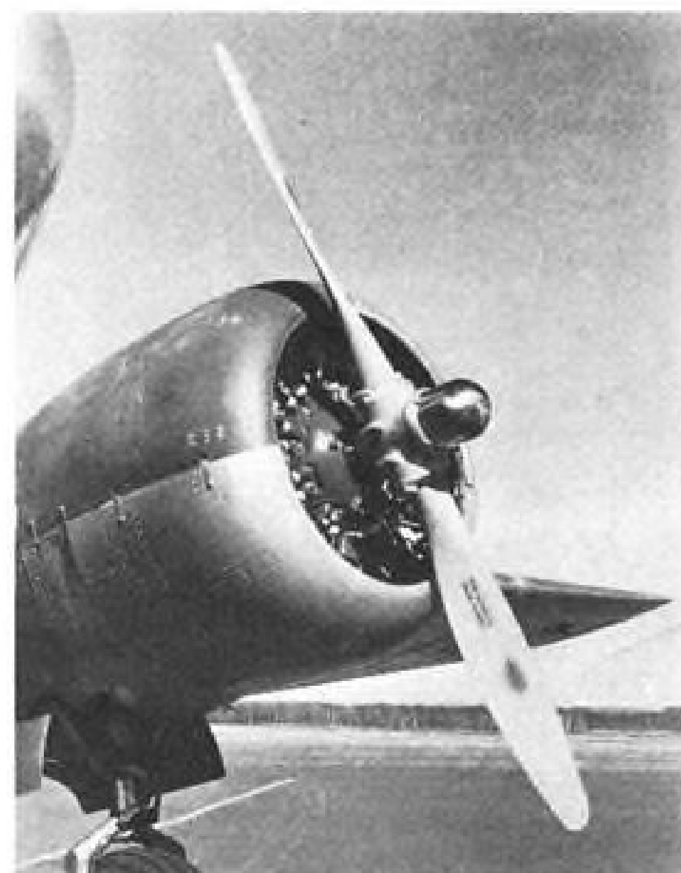
Smaller Hydromatic: Hamilton Standard Propellers division of United Aircraft Corp. has put into quantity production this "baby" version of its widely-used Hydromatic prop. It ranges in size from eight to ten feet in diameter.
