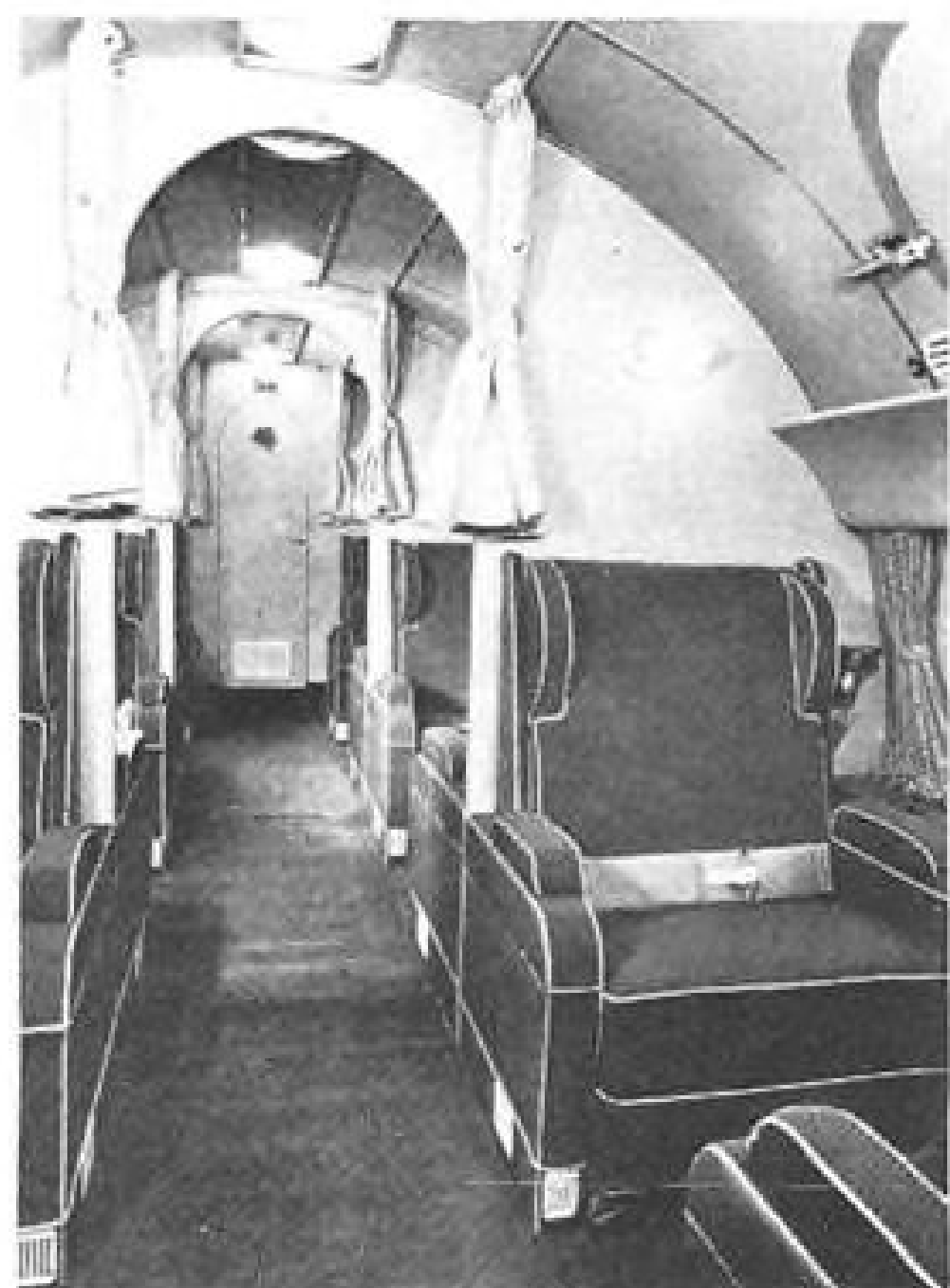
"Tudor I" Cabin: Interior of the cabin in the Tudor I BOAC will use in North Atlantic service. Air conditioning inlet louvers are near the floor in the chair armrests. Not shown are additional louvers in the side walls of each compartment. Outlets are slots around reflectors for the roof lights.
