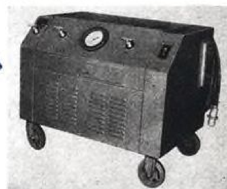
Model PE3-8 — An electric motor-driven portable hydraulic test machine for line testing the performance and operation of complete airplane hydraulic systems up to 3,400 psi at 8 gpm flow. Also supplied with flows up to 20 gpm at 3,400 psi (Model PE3V-20V). Both are supplied also as gasoline-engine driven.
