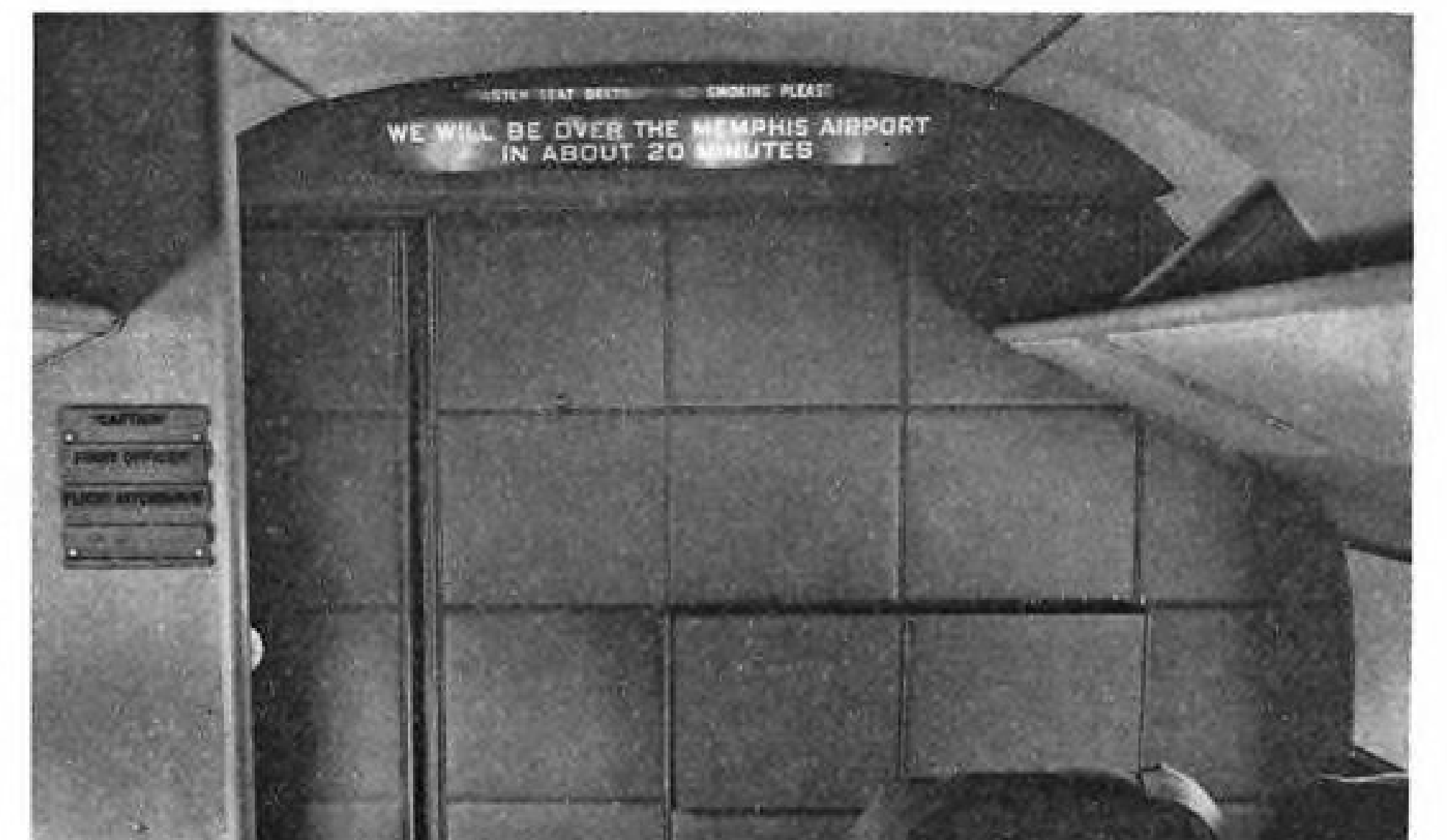
Telling the Passenger: So Chicago and Southern passengers may know their whereabouts, flight information signs like that shown here have been installed in newly converted C&S DC-4's. Picture of cabin's front bulkhead shows (left) door leading to galley, through which pilot compartment is reached.
