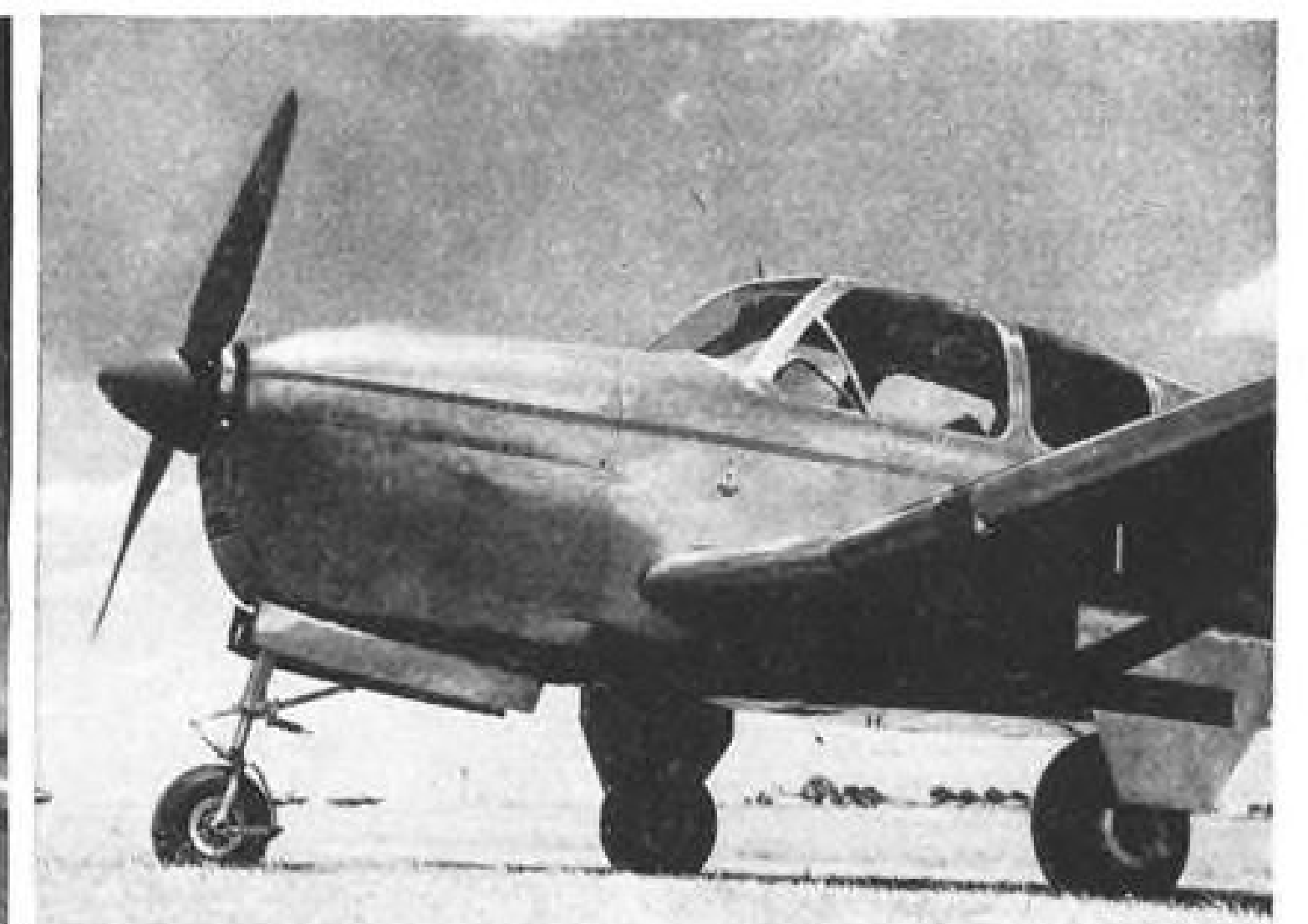
retractable, tricycle gear uses large size tires for rough fields. Nosewheel is free-swivelling with side bracing, hydraulic shimmy-dampener, and mud scraper.
