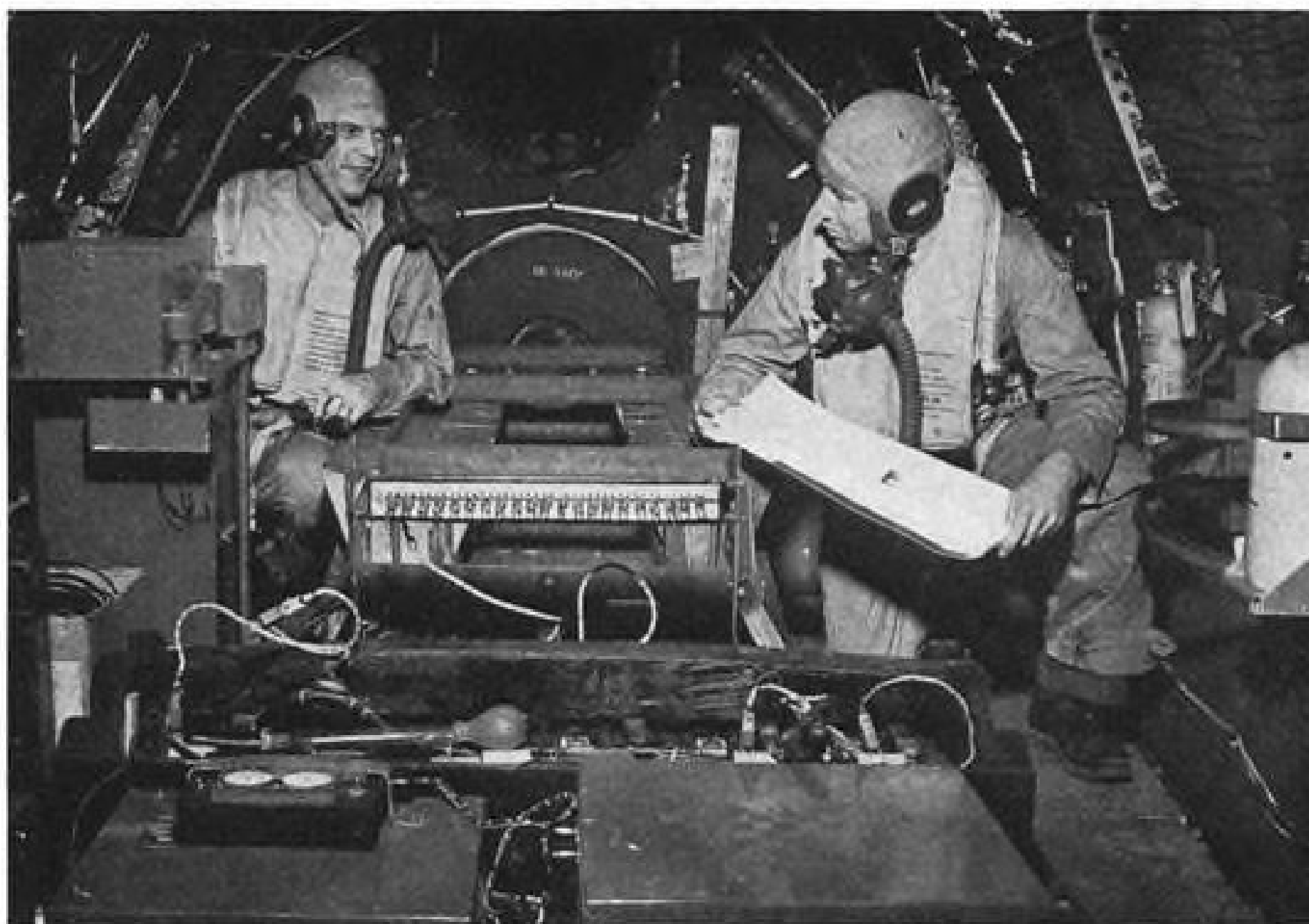
Cosmic Ray Recorders: Cosmic rays found at altitudes ranging from 5,000 to 35,000 ft. are measured on banks of Geiger counters (center) in a converted B-29 bomber which is being used under sponsorship of National Geographic Society, AAF and Bartol Research Foundation. Ed Kurtzner and Peter Morris operate the apparatus.
