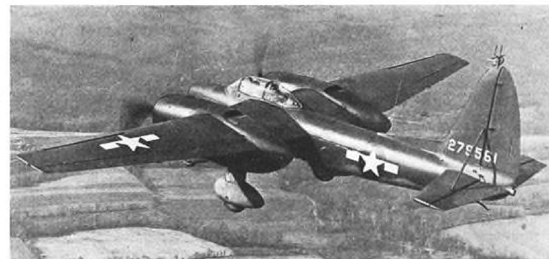
Kaiser Robot Attack Plane: First flight picture of the XBQ-1 Kaiser Fleetwings Inc. experimental, radio-controlled attack plane developed for the AAF during the war. Note radio control antenna on vertical stabilizer.
