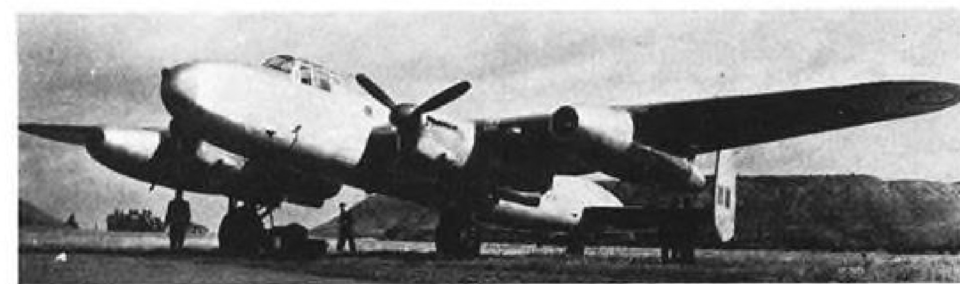
Combination Power: Exhibited at the British aircraft show was this Lancastrian (transport version of the bomber) with two Merlin reciprocating engines and, in outboard positions, two Rolls-Royce Nene jet engines. With all four engines operating, this aircraft attained more than 300 mph. With only the two jets furnishing power, it flew between 250 and 280 mph. (McGraw-Hill photo)
