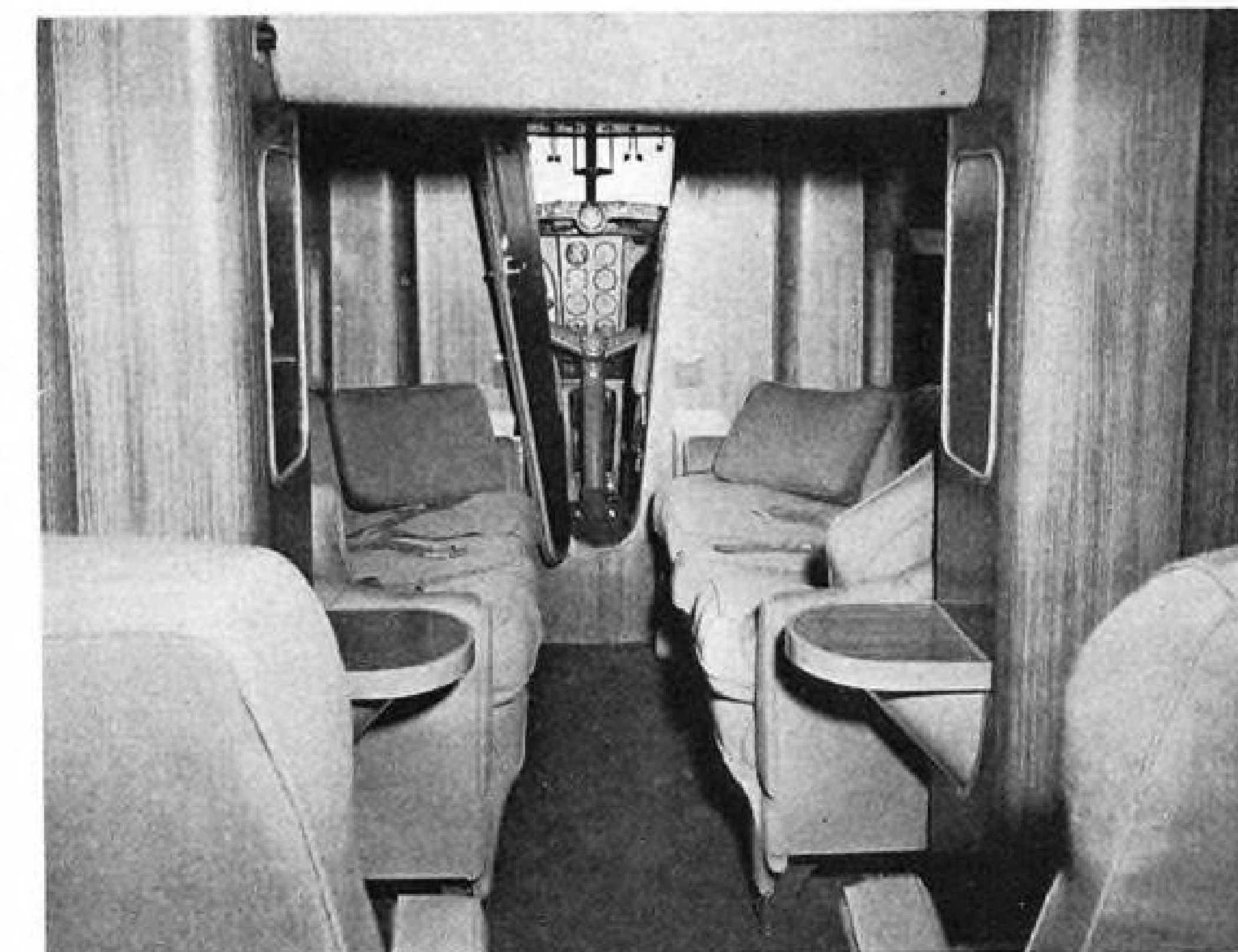
Amphibian Interior: Looking forward to pilot's compartment, interior view of Grumman Mallard amphibian's luxurious passenger cabin shows facing divans and airline type seats, accommodating 8 passengers, plus crew of 2. (Martin and Kelman photo)
