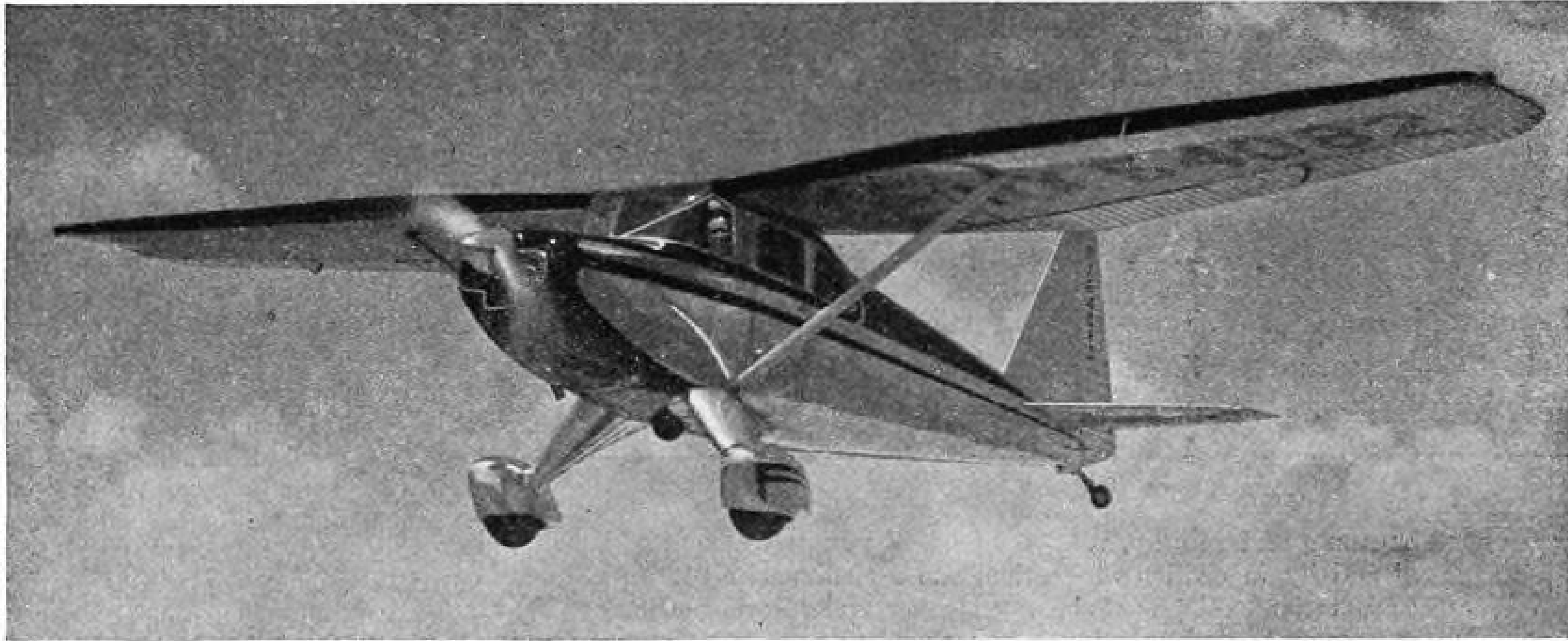
Exceptional stability, fast climb, and high speed are stated to feature Lycoming-powered Weatherly-Campbell Colt. Dual taper of wings is particularly noticeable in this flight view.
