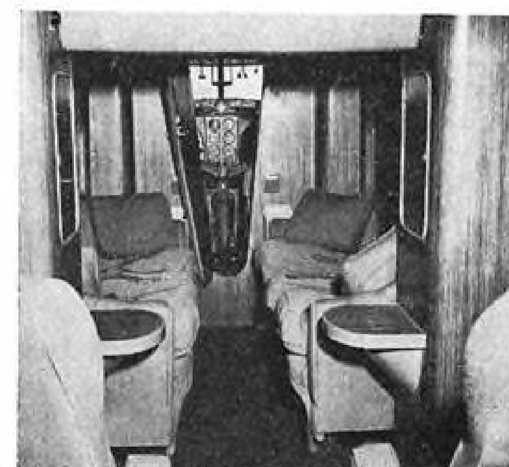
Mallard cabin interior looking forward from aft compartment which has four seats facing forward. Thermostat at upper left controls cabin temperature; panel at right encloses food compartment. Mid-sections of divan-type seats are easily removable to set up tables. (Martin & Kelman photo)
