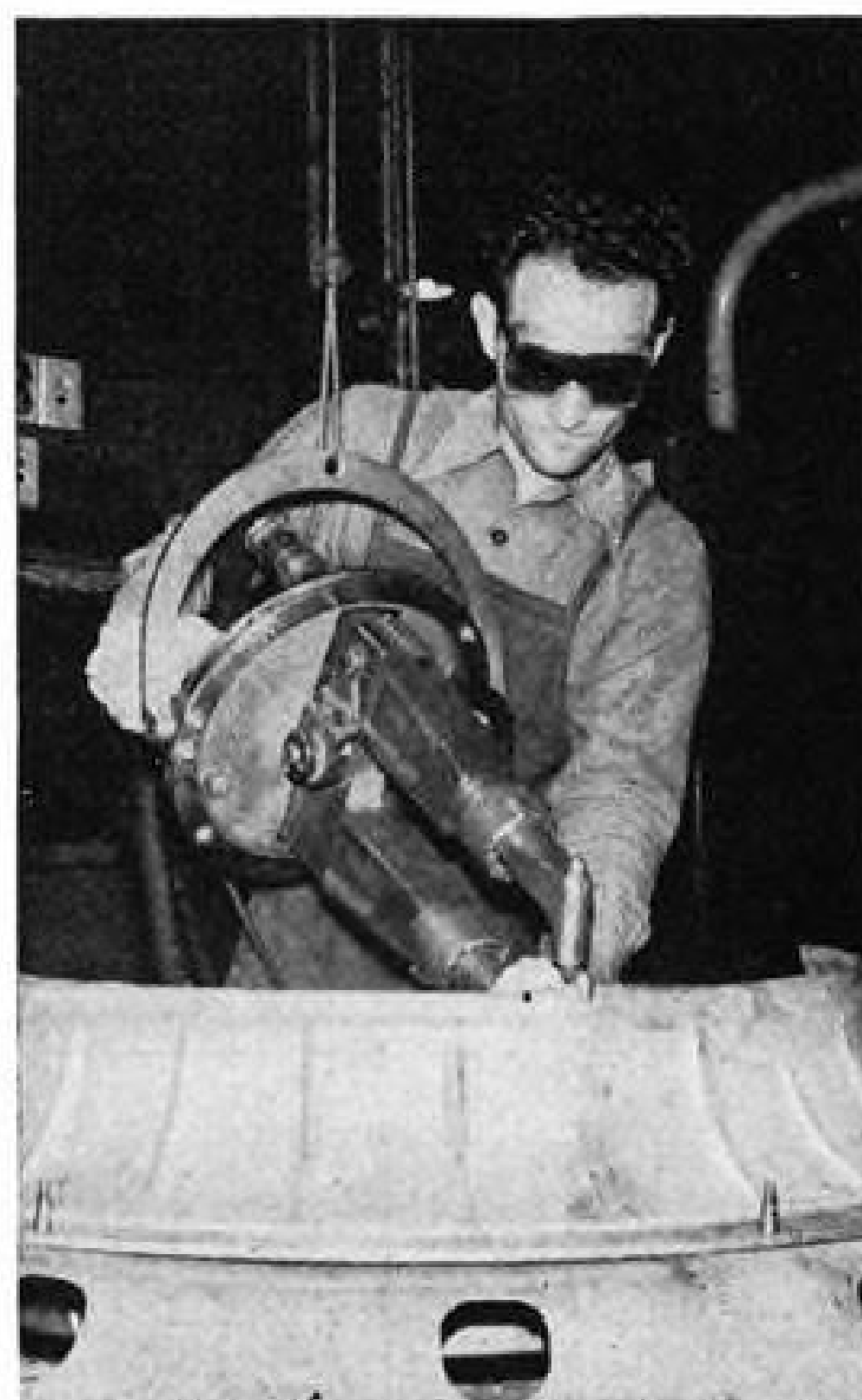
Counterbalanced air-operated water-cooled spotwelder seen here is used at Ryan Aeronautical Co. for reaching high restricted locations.
