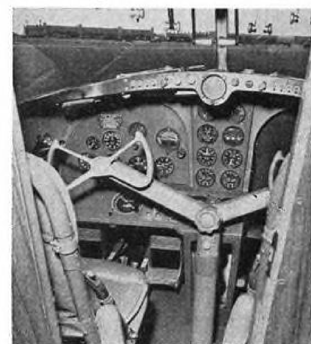
Cockpit of Grumman Mallard, showing dual radio controls installed on panel at windshield base, also throttle, flap, and landing gear controls suspended from cockpit roof. Co-pilot's wheel is quickly detachable for easier access to forward hull compartment. (Martin & Kelman photo)
