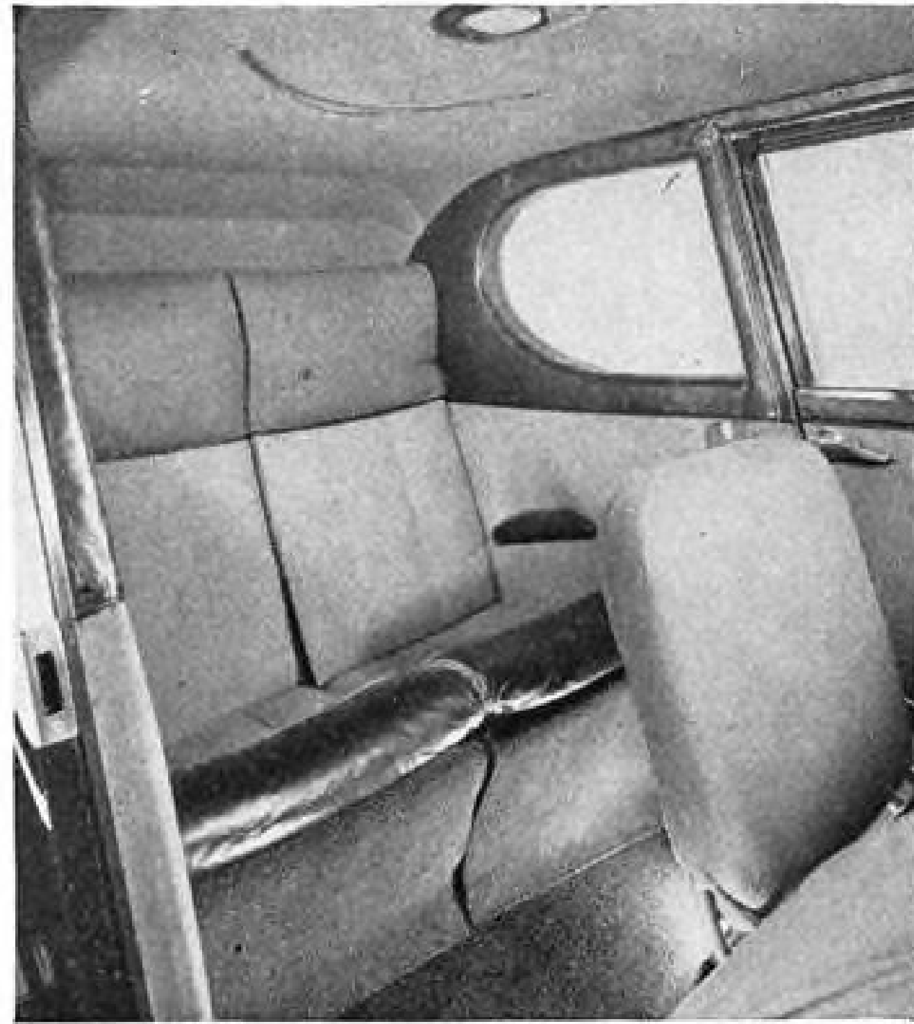
Rear seats have padded hair and cotton cushions with Koroseal covered knee rolls and trim. In addition to fitting dual mufflers to 150-hp. Franklin, further cabin noise insulation is provided through use of 120-sq. ft. of Fiberglas blankets, weighing but 2½ lb. Note dome light and speaker in roof. Back seats can be readily removed and 600 lb. of cargo carried.
