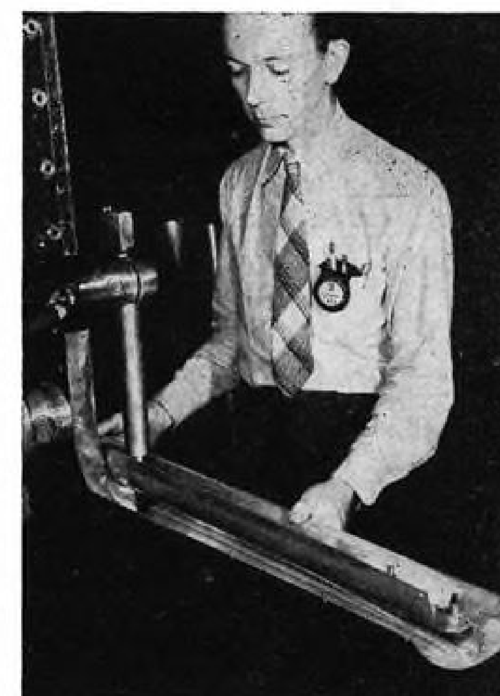
Ryan-designed electrodes are used to spotweld this somewhat inaccessible aluminum vane. Bottom electrode is copper, backed with steel for high strength.
