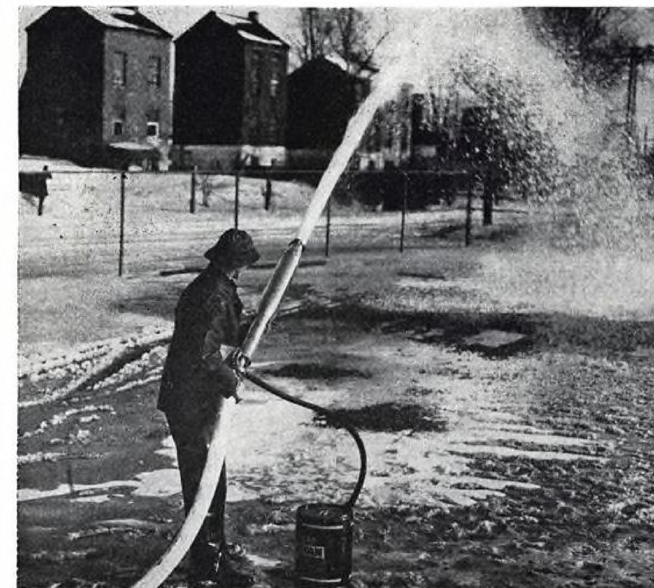
National Aero-O-Foam unit is designed to be handled by one-man. Chemical is drawn up from can by suction and is mixed with water at butt of special nozzle held by operator. It's stated that one 5-gal. container can thus be diluted to make approximately 800-gal. of foam.
