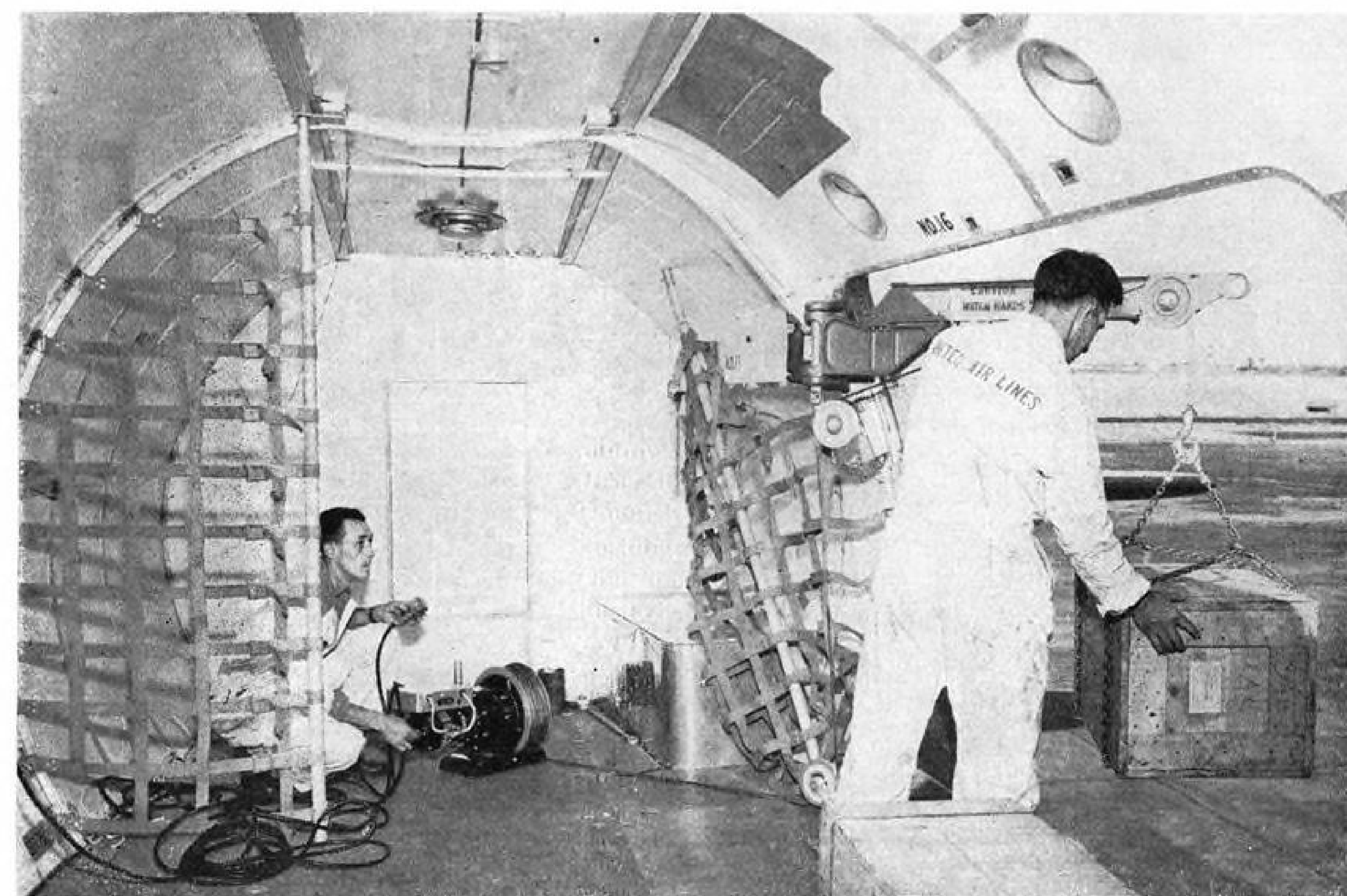
This interior view of UAL's Cargoliner 230—Douglas DC-4—shows thermo-sealed curtain for shutting off aft section of plane to provide 300-cu. ft. refrigerated section. Movable electric winch, seen on floor
