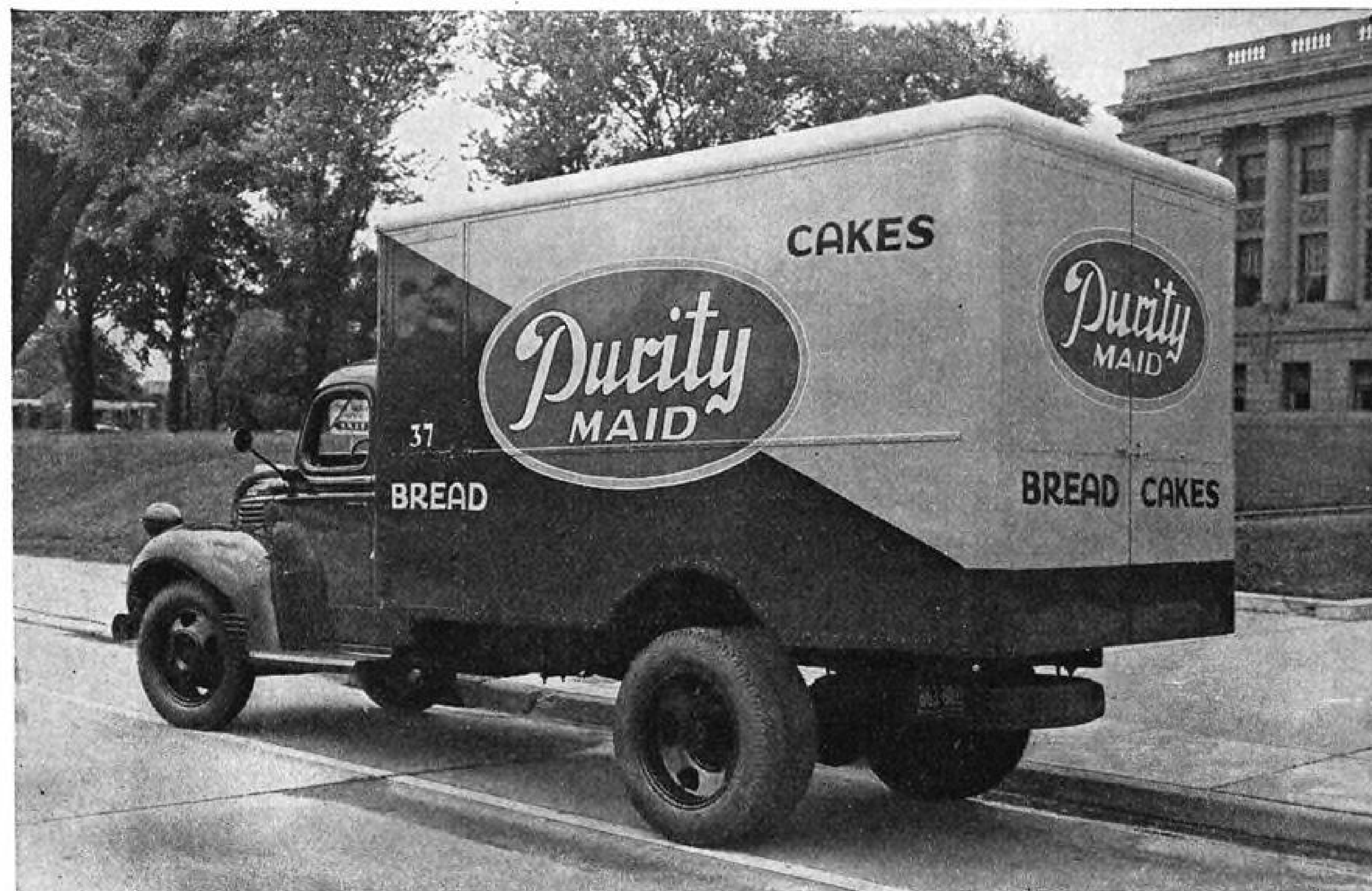
Magnesium alloy body built by Purity Baking Co. from Revere sheet and standard shapes. Outside dimensions are 139 1/4" long, 80 1/4" wide, and 76" high. Weight of body, including interior tray racks to hold 2150 loaves of bread, is 1060 lbs. in magnesium compared to 2300 lbs. in steel.
