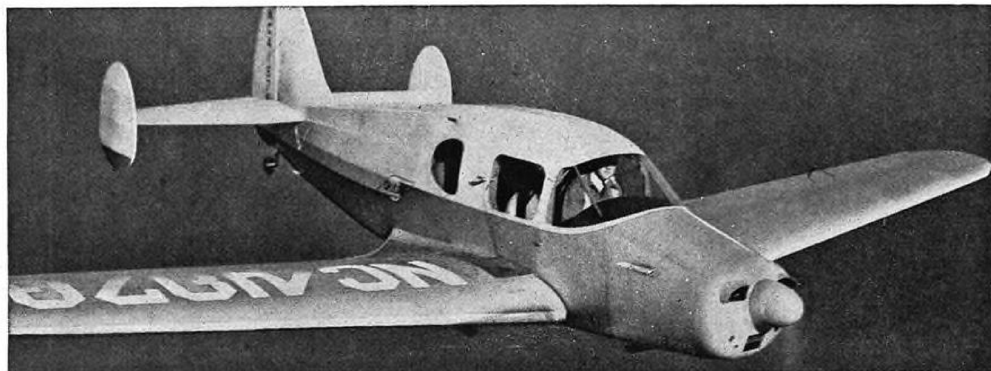
New Bellanca "Cruisair" . . . 150 H.P., 4-place model. Factory-equipped with an Aeromatic, it does 169 M.P.H.
