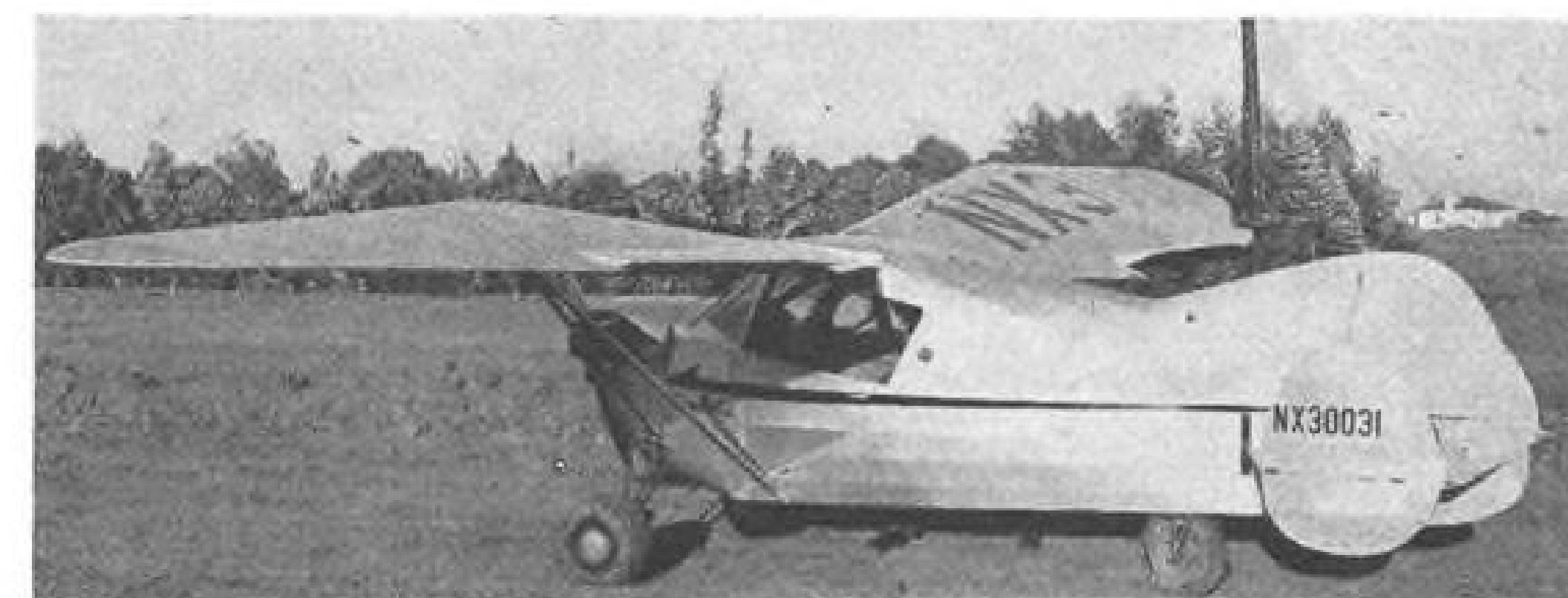
Variable Incidence Wings: Ready for flight after 15 minutes of conversion with wrench, screwdriver, hammer and drift punch, the Los Angeles-built Plane-Mobile has its right pivoted wing section set at increased incidence as if to make a climbing left turn. (Aviation News photo)
