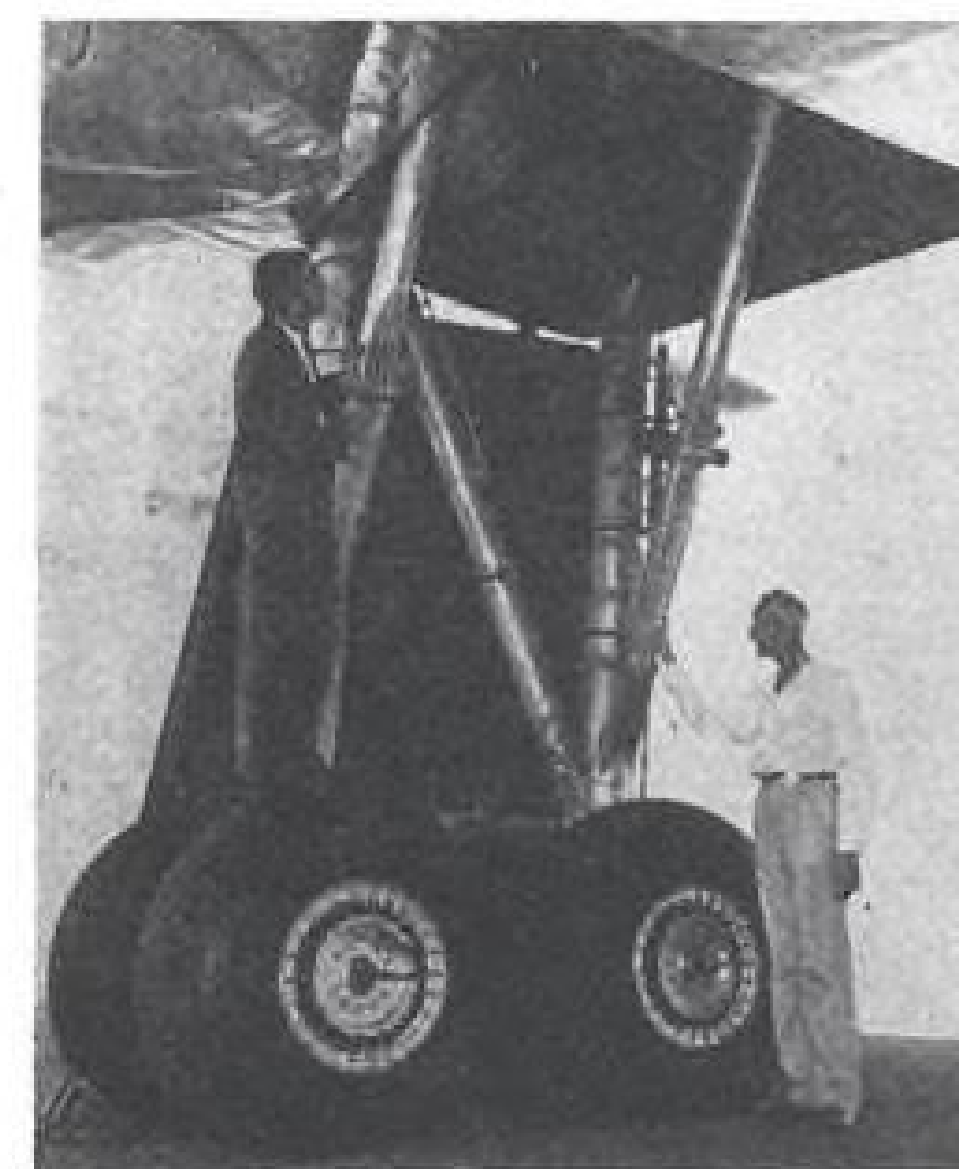
Daddy Long-Legs: One of the main wheel units of the Lockheed Constitution, 92-ton Navy transport which made its initial flight last week. Each of the four 50-inch diameter wheels has its own brake. Because of the rotovane self-starting tires, a smaller and lighter landing gear assembly is needed than would be the case if single or double wheels were used.
