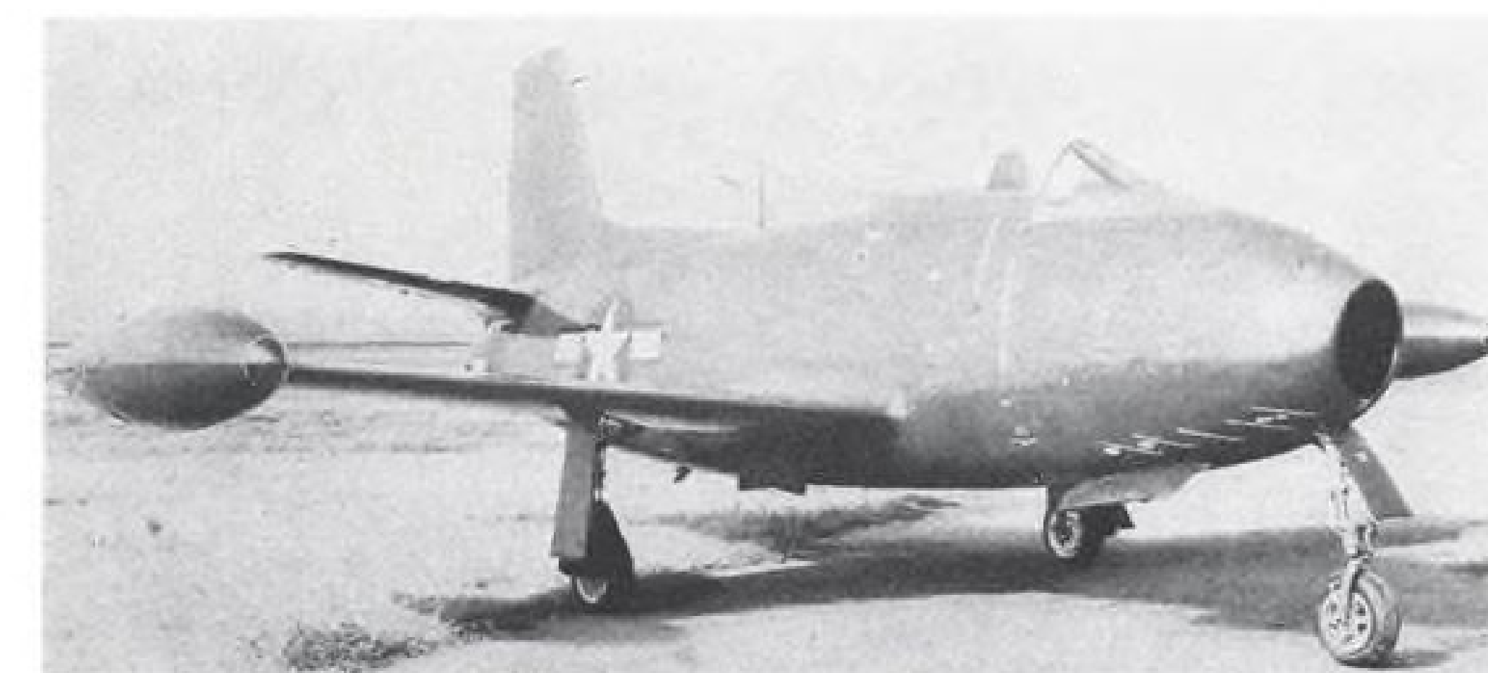
North American's Navy Jet Fighter: First photo of the new North American jet fighter, XFJ-1, built for the Navy and now undergoing test flights at Muroc Lake, Calif. Powered by a General Electric TG-180, this plane is classed by the Navy as "better than 500 mph." (Navy photo)
