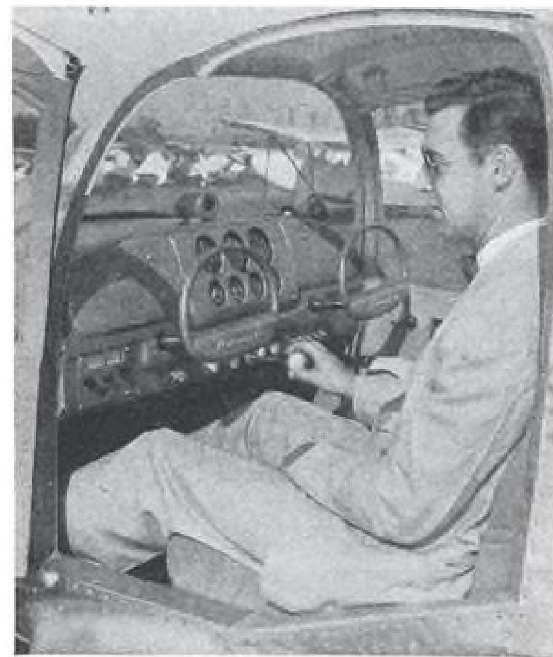
Aeronca's Two-place Chum: Centralized arrangement of instruments on panel and new safety-type control wheels are attractive interior appointments of new simplified-control Aeronca Chum. First all-metal
