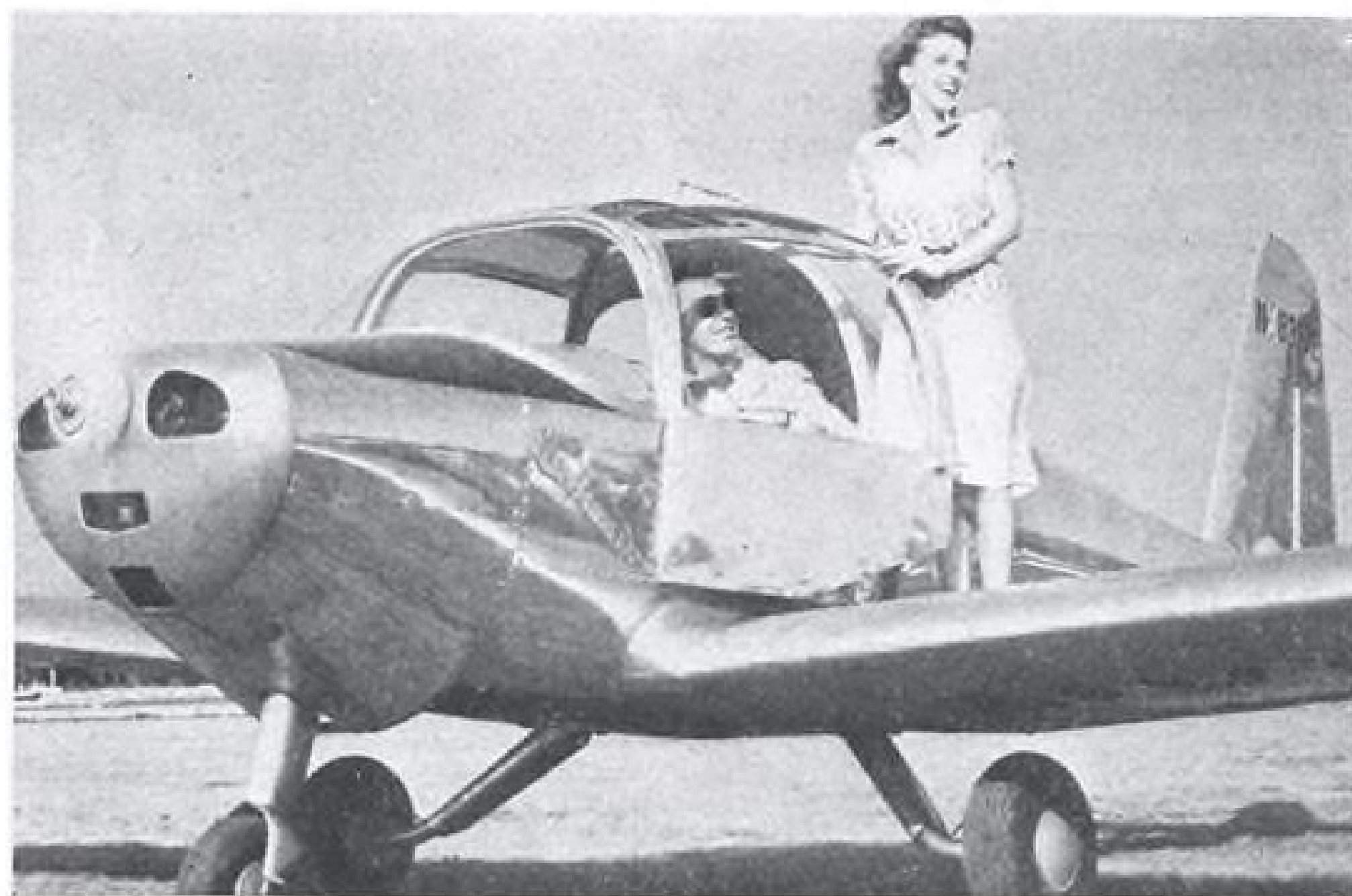
Aeronca plane, the Chum has fixed tricycle landing gear with unusually wide tread, giving good ground-handling characteristics. Power plant is Continental engine with fuel injection.
