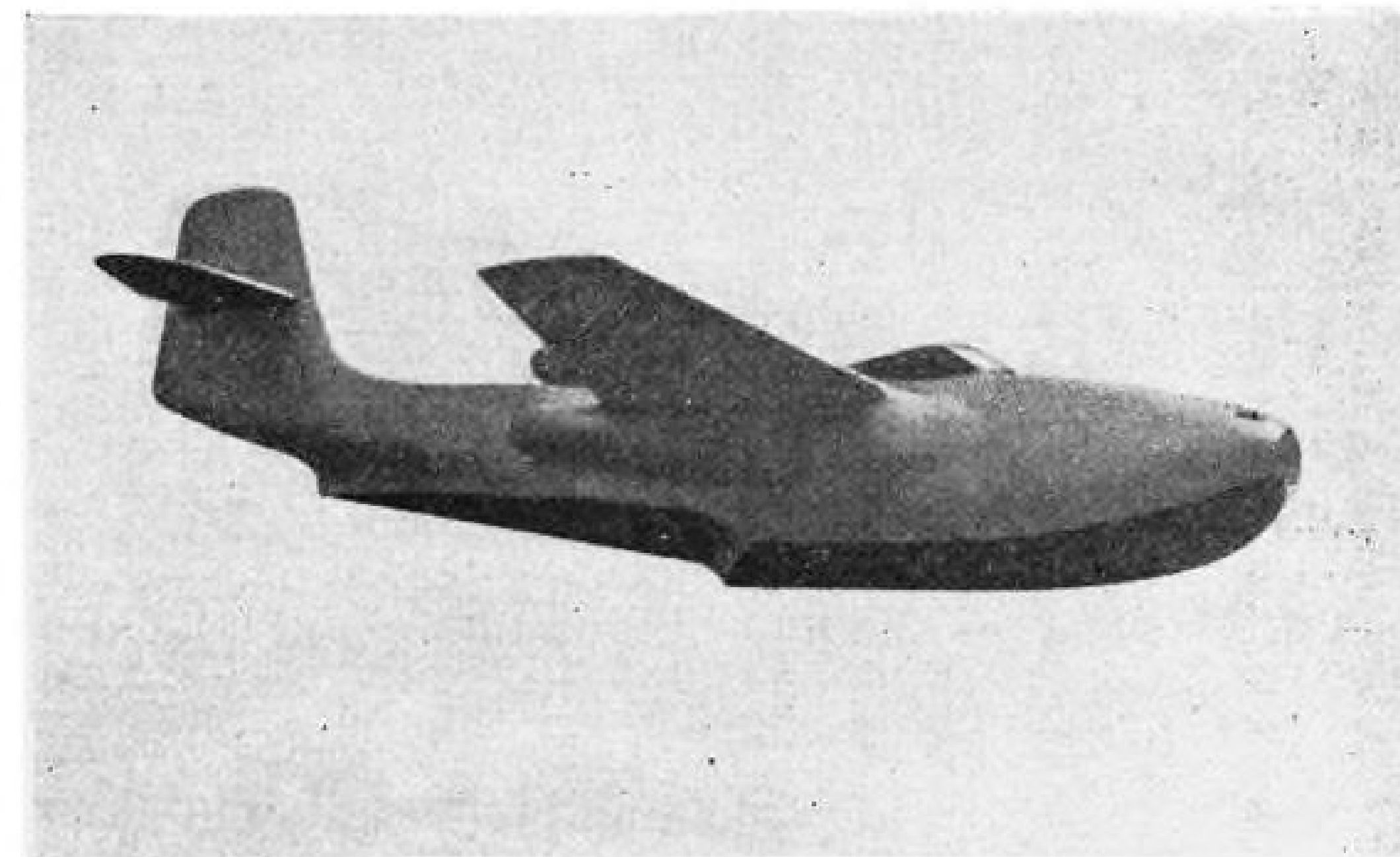
Twin Jet Flying Boat Fighter: Model of Saunders-Roe SR/A1 design which is to be powered by two Metro-Vickers F2/4 axial flow jets of 3,500 lb. static thrust each. A high wing single-seat flying boat fighter, the SR/A1 will have pressure cabin and pilot ejection equipment, semi-retractable wing floats. Tank tests are said to show air intake at bow is free from adverse spray effects under normal operating conditions; a trap would prevent entry of sea water under abnormal circumstances.
